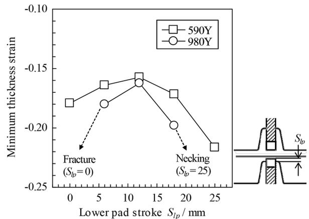
Fig. 4 Improvement of flange-up formability by developed method
