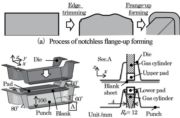
(a) Process of notchless flange-up forming
