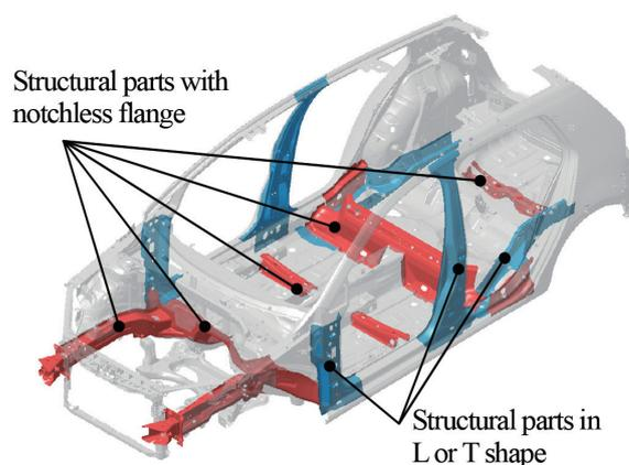
Fig. 1 Body structural parts to which developed forming methods are applicable
