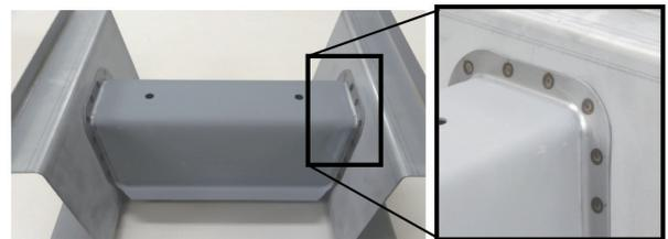
Fig. 9 Simulated cross member of UHSS sheet having flange joints without notches
