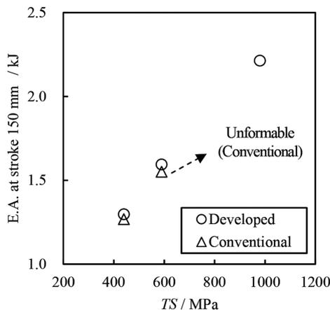
Fig. 15 Improvement of crash performance of structural parts formed by Free Bend Sheet Forming
