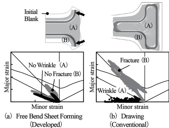
Fig. 12 Mechanism of formability improvement by Free Bend Sheet Forming
