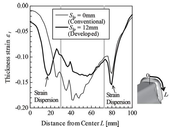
Fig. 5 Improvement of strain dispersion by developed method
