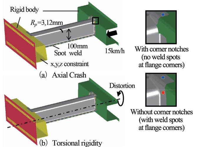
Fig. 7 Performance evaluation model simulating actual auto-body parts
