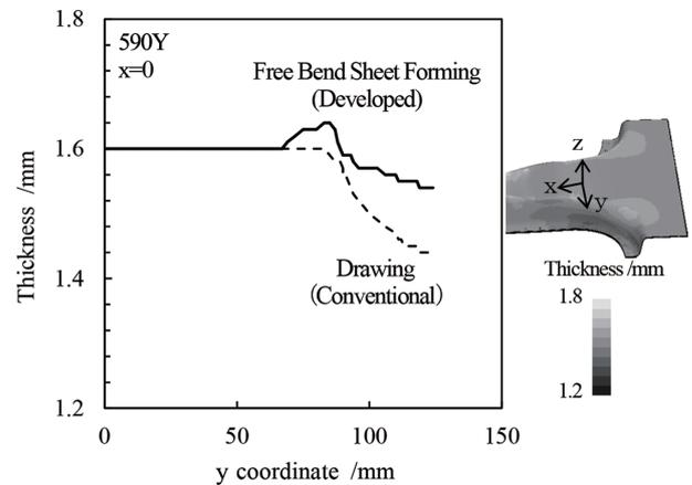
Fig. 16 Suppression of thickness decrease by Free Bend Sheet Forming
