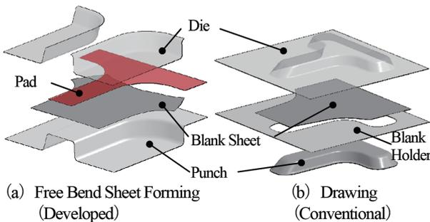
Fig. 11 Comparison between developed and conventional forming method
