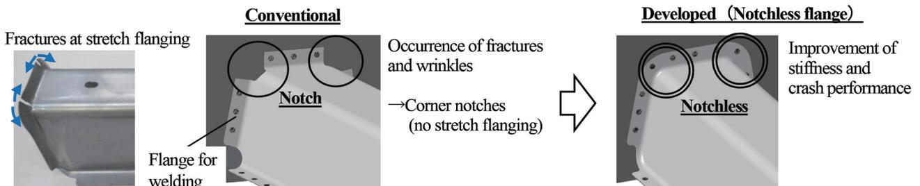
Fig. 2 Conventional problems solved by developed forming method
