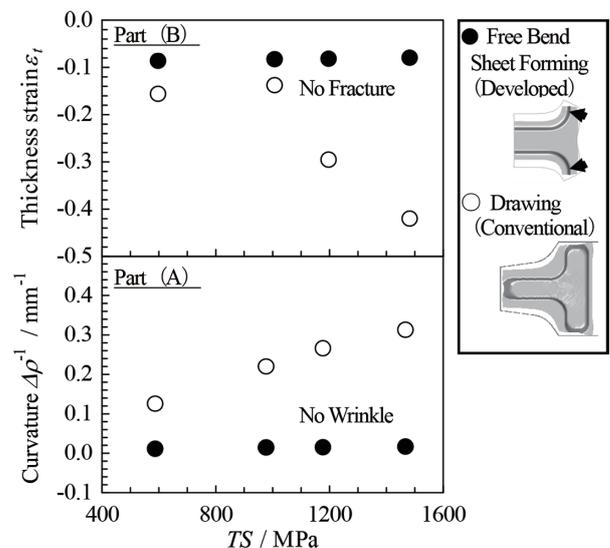
Fig. 13 Improvement of formability by Free Bend Sheet Forming
