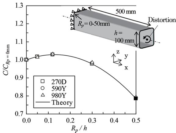
Fig. 6 Effect of sectional shape on torsional stiffness
