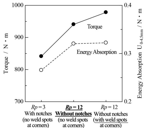
Fig. 8 Performance improvement by notchless flange and shape optimization
