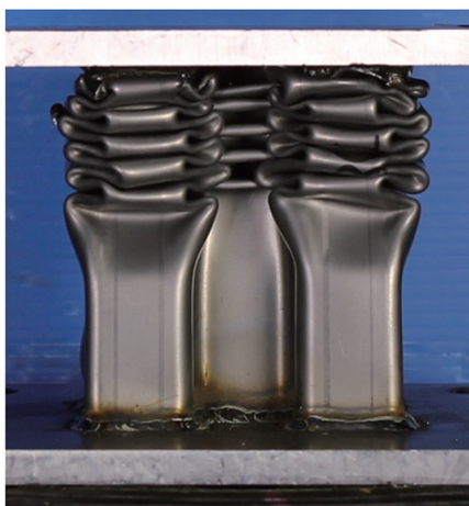
Fig. 7 Axially crushed specimen of 1180 MPa high strength steel for energy absorbing parts
