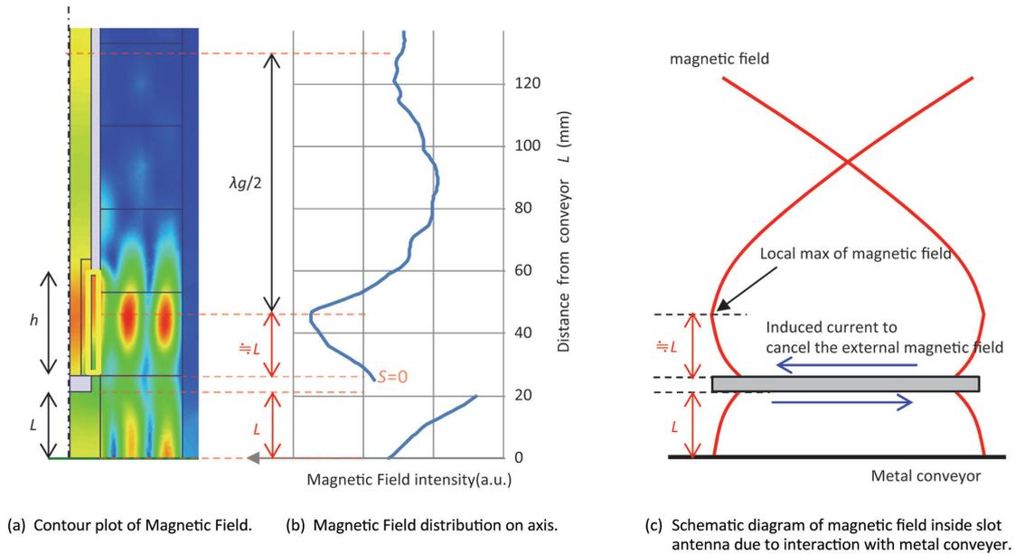
Fig. 5 Calculated magnetic field distribution inside slot antenna inserted into agglomerate layer
