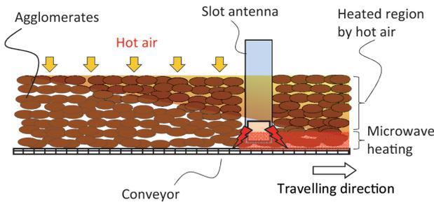
Fig. 1 Schematic diagram of microwave heating equipment for the band dryer
