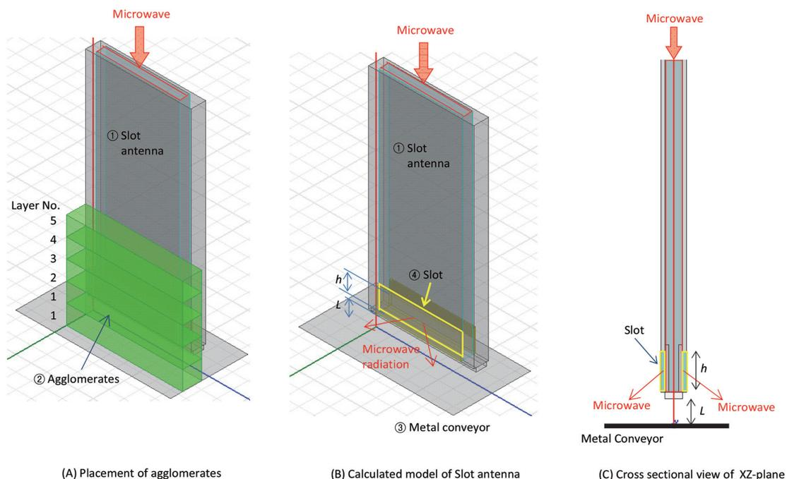
Fig. 4 Geometry of the numerical simulation model
