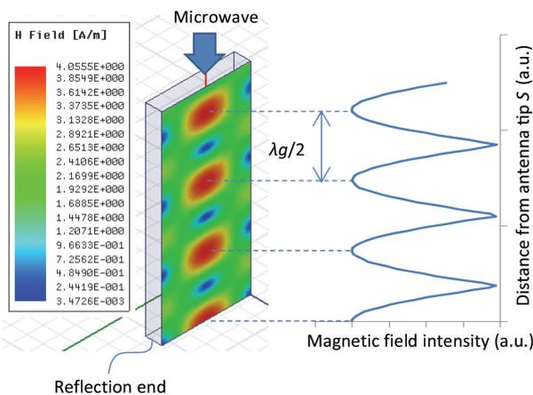
Fig. 3 Magnetic field distribution of E-plane inside a slot antenna
