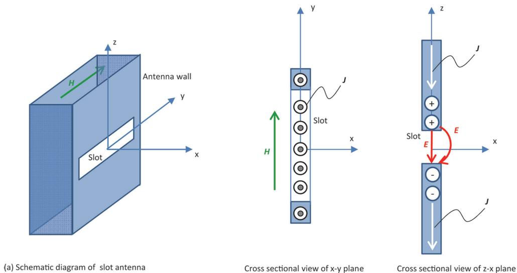
Fig. 2 Microwave radiation from a slot antenna
