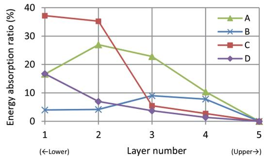
Fig. 7 Energy absorption ratio at different layers
