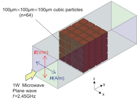
**Fig. 8 Geometry of the numerical simulation model**
