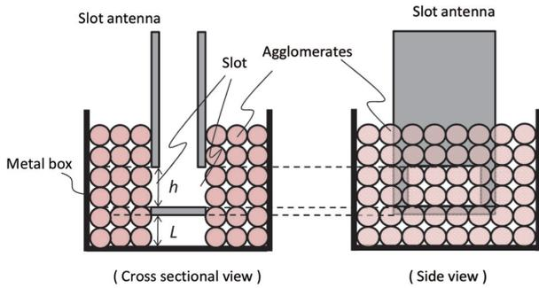
Fig. 6 Experimental setup of microwave heating of agglomerates using slot antenna
