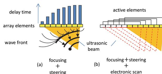
Fig. 1 Phased array ultrasonic testing technique
