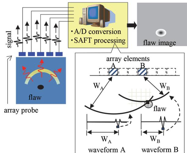
Fig. 4 Synthetic aperture focusing technique
