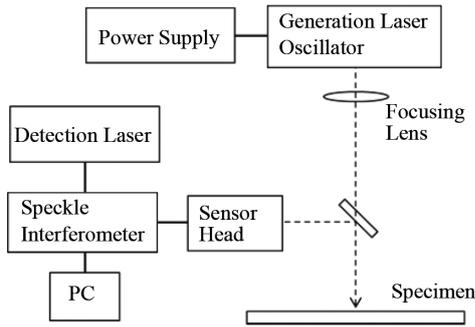
Fig. 7 Schematic diagram of the stress measurement system
