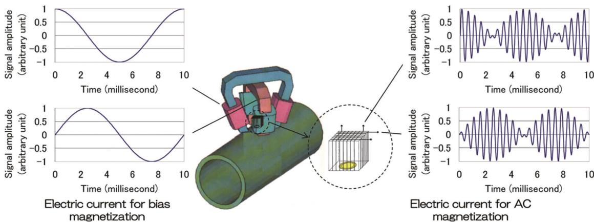
Fig. 14 Schematic configuration of SMaRT device
