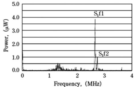
Fig. 10 Power spectrum of the output signal from a sample with stress (15 MPa)
