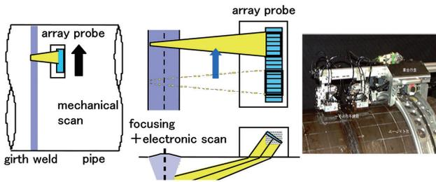
Fig. 2 Ultrasonic testing system for girth weld joints
