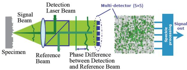
Fig. 8 Principle of ultrasonic stress measurement with interferometer
