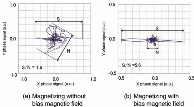
Fig. 16 Improvement of SN ratio (specimen: 0.25%C steel pipe)
