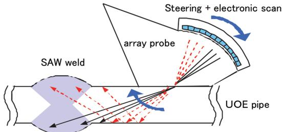
Fig. 3 Ultrasonic testing of UOE pipe seams using array probe
