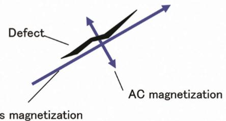
Fig. 13 Optimum AC magnetization and bias magnetization for flaw detection
