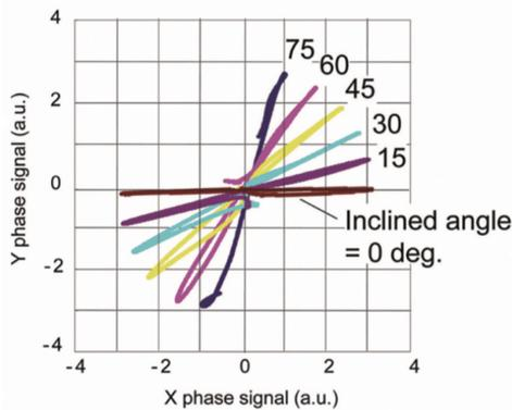
Fig. 15 Relationship between signal wave form and crack angle by SMarT
