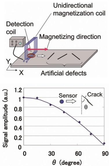
Fig. 12 Relationship between signal amplitude and crack angle
