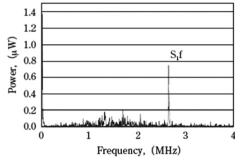
Fig. 9 Power spectrum of the output signal from a sample without stress
