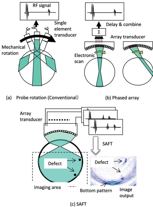
Fig. 6 Ultrasonic testing technique for cylindrical products
