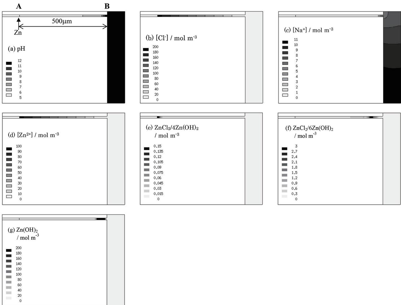
Fig. 8 Results of numerical analysis under paint film near shear cut edge of galvanized steel sheet in NaCl 500ppm solution<sup>9)</sup>
