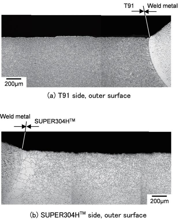
tion heating, it was made possible in the present test to heat SUPER304H™, T91 and the weld metal to substantially the same temperature by adequately designing the shape of the induction coil. In addition, by adjusting the air blow, the temperature of the joint and adjacent portions was kept nearly even during cooling, and as a result, desired heat cycles were applied to the joint and the adjacent portions.
