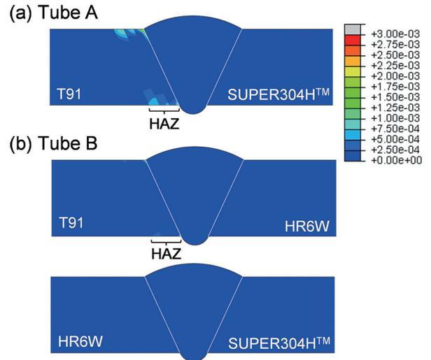
Fig. 8 Calculated distribution of creep strain near dissimilar welded joints
