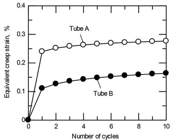
Fig. 9 Relationship between equivalent creep strain and number of cycles at the weld toe in T91
