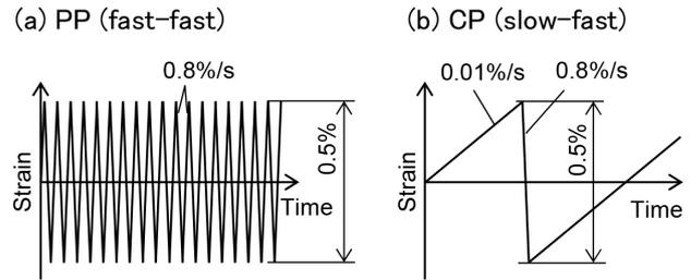
Fig. 2 Strain waveforms for the creep-fatigue test
