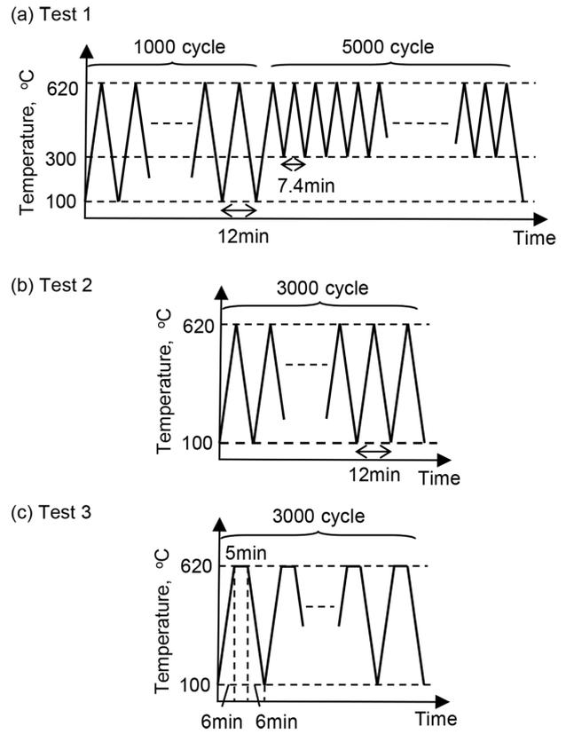
Fig. 4 Temperature cycles for the thermal fatigue test
