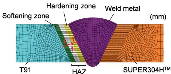
Fig. 7 FE-model of dissimilar welded joint
