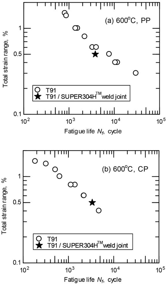
Fig. 3 Comparison of creep fatigue life of dissimilar welded joints under different strain waveforms
