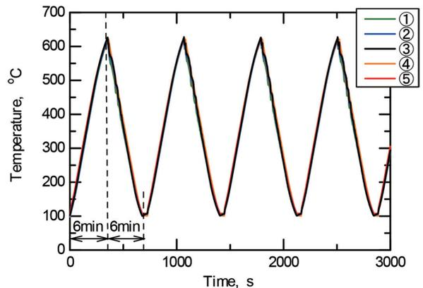
Fig. 5 Temperature measurement at different positions of dissimilar welded joint during heat cycles
