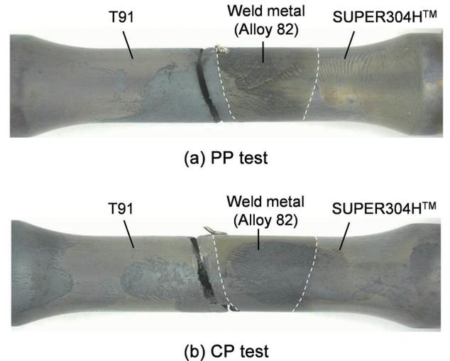
Photo 1 Appearance of the specimens after the creep-fatigue test
