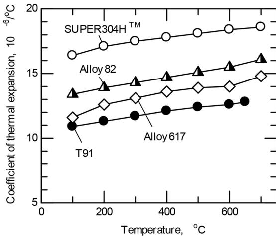
Fig. 1 Coefficient of thermal expansion of SUPER304H™ and T91
