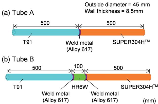
Fig. 6 Dissimilar welded tube of SUPER304H™ for FE-analysis
