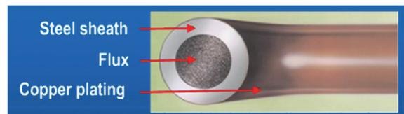
Fig. 8 Schematic image of cross section on seamless type flux cored wire
