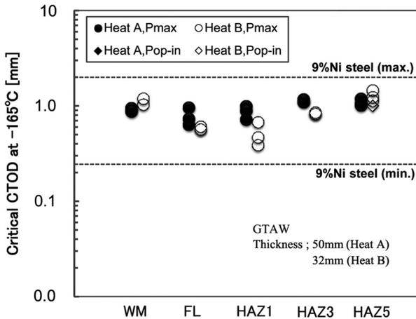
Fig. 11 CTOD test results of welded joints
