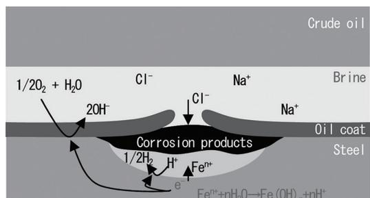
Fig. 6 Summarized process and mechanism of localized corrosion on COT bottom plate
