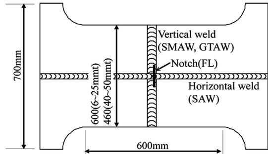
Fig. 12 Specimen of cross weld notch wide test
