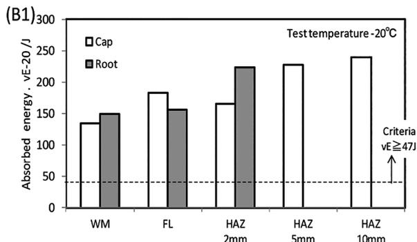
Fig. 16 Charpy impact test results of welded joints by high arc energy welding
