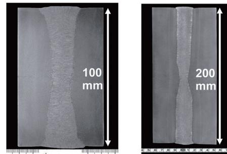
Fig. 4 Macrostructure of welds 100 mm and 200 mm thick with four-electrode VEGA® welding process
