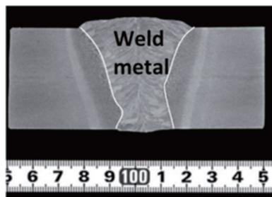
Fig. 15 Example of macro sections by high arc energy welding
