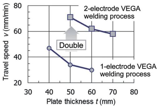
Fig. 2 Comparison of travel speed with single- and two-electrode VEGA®
