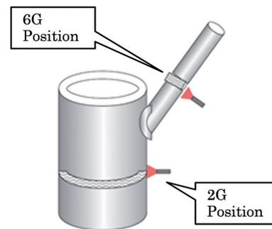
Fig. 7 Example of welding positions required in the TOKYO SKYTREE®
