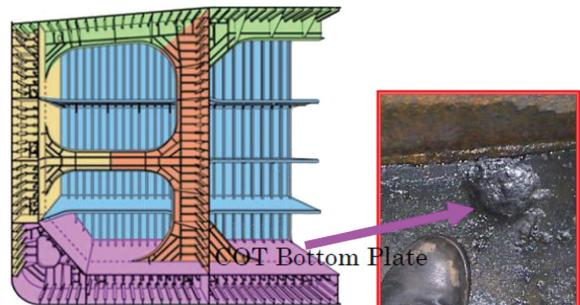
Fig. 5 Example of pit corrosion on COT (Crude Oil Tank)
