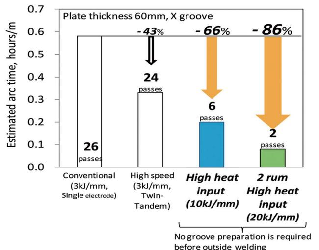
Fig. 14 Advantages of high heat input SAW in arc time
