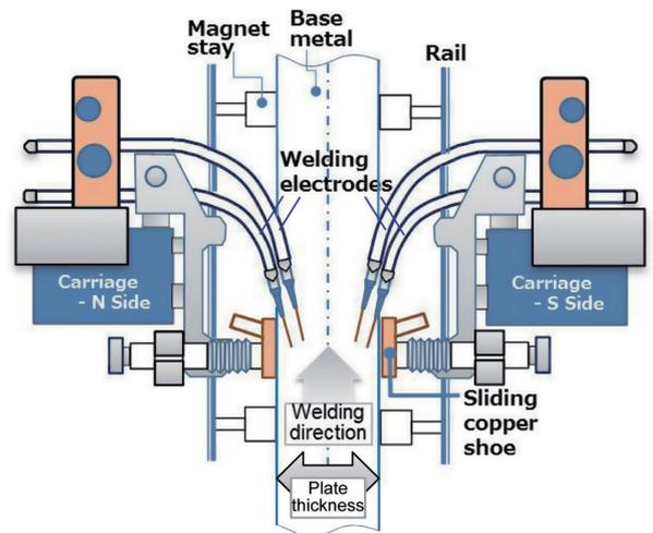
Fig. 3 Schematic diagram of four-electrode VEGA® welding process
