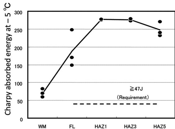
Fig. 9 Charpy impact test results of welded joints on SBHS500 steel by high arc energy SAW
