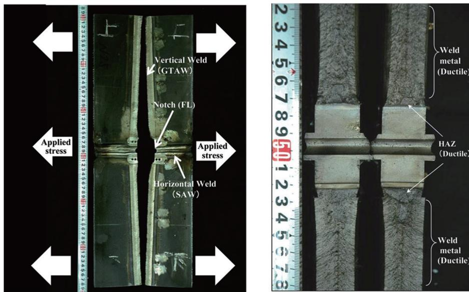
Fig. 13 Fracture path and fracture surface of cross weld notch wide test (Heat A, 25 mm)
