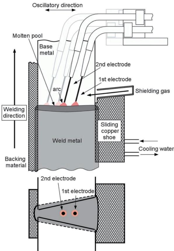
Fig. 1 Schematic diagram of two-electrode VEGA® welding process
