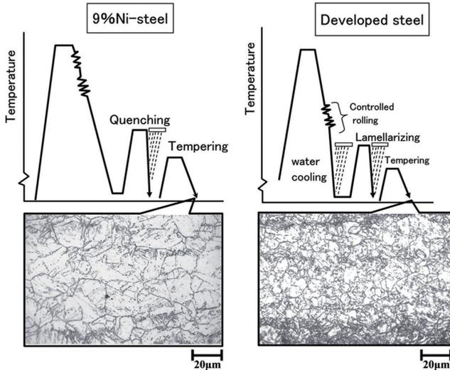
Fig. 10 Production process and microstructure
