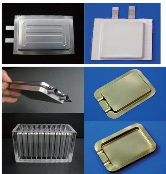
Fig. 7 Packs of laminated stainless steel foil formed by pressing without lubricants
