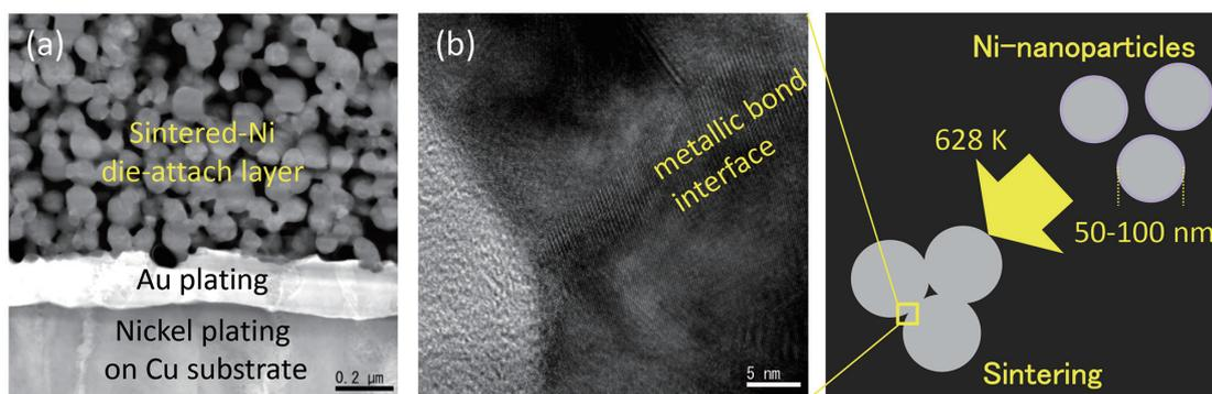
Fig. 6 Cross sectional TEM images of (a) Joint of Ni nanoparticle layer and Ni/Au plated substrate, (b) Ni nanoparticle layer, after heating at 628 K
