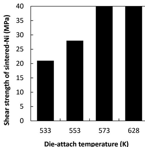
Fig. 5 Shear strength of sintered-Ni layer after heating at 533, 553, 573 and 628 K
