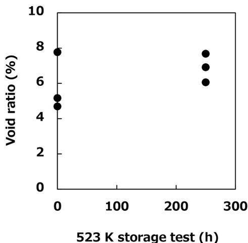
Fig. 8 Change in void ratio of die-attach layer of sintered Ni particles after storage at 523 K
