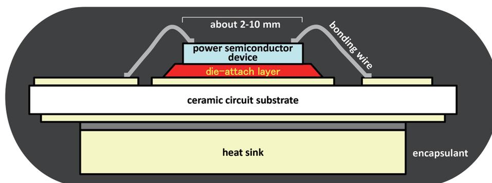
Fig. 1 Schematic cross-sectional illustration of a typical power module
