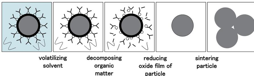
Fig. 3 Schematic illustration of the die-attach process using nano-particles
