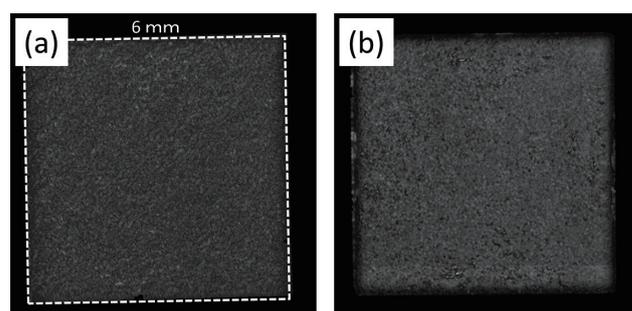
Fig. 7 SAT images of sintered-Ni die-attach samples (a) Before and (b) After 200 cycles of 233/273 K TCT
