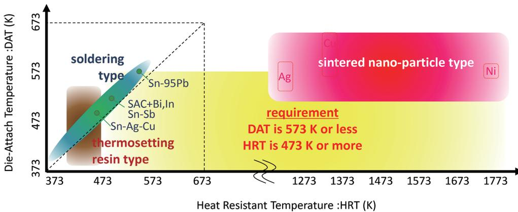
Fig. 2 Relationship between heat resistant temperature and die-attach temperature
