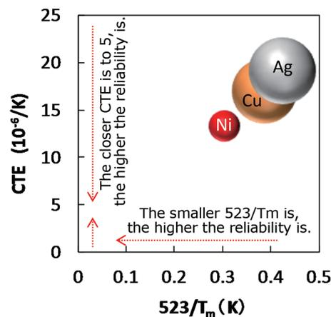
Fig. 4 Thermal properties of Ag, Cu and Ni
