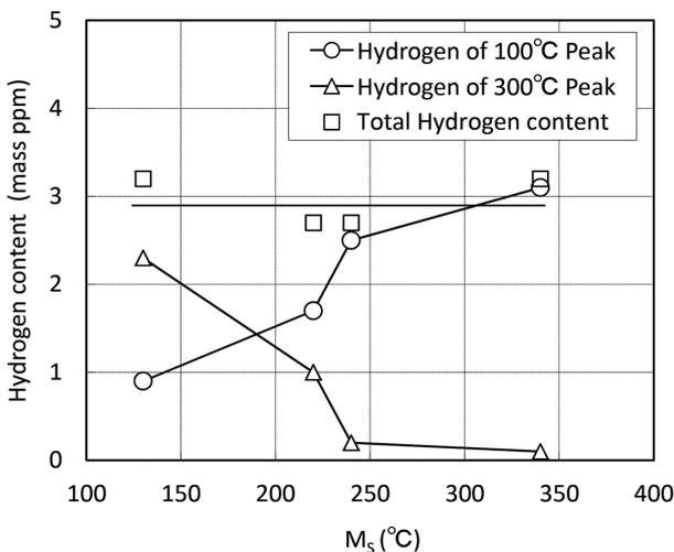
Fig. 4 Effect of carbon content on the amount of hydrogen in steel that annealed in hydrogen atmosphere followed by quenching<sup>11</sup>
