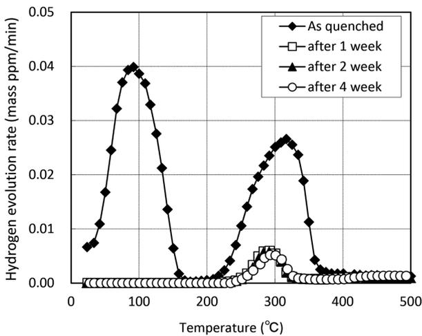
Fig. 3 Changes in TDA curves with aging at room temperature of 0.82 mass% C steel annealed in hydrogen atmosphere followed by quenching<sup>12</sup>
