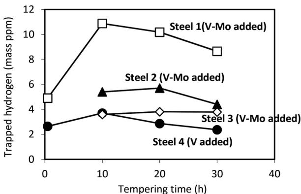
Fig. 8 Hydrogen trapping capacity of V-Mo added steels for various tempering time<sup>15)</sup>
