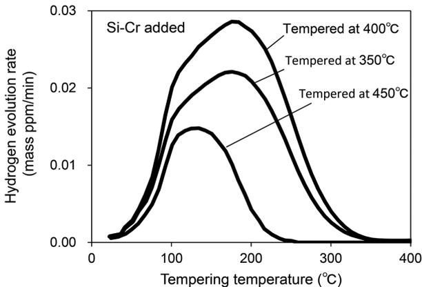
**Fig. 11** Hydrogen evolution rate curves of Si-Cr added 0.6%C steel tempered at various temperatures<sup>17)</sup>
