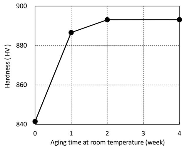
Fig. 6 Changes in Vickers hardness with aging at room temperature of 0.82 mass% C steel annealed in hydrogen atmosphere followed by quenching<sup>12</sup>
