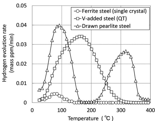
Fig. 1 Hydrogen thermal desorption analysis (TDA) curves for steels with various hydrogen trap
