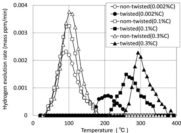
Fig. 7 Changes in TDA curve of low carbon steel by torsion processing<sup>13)</sup>
