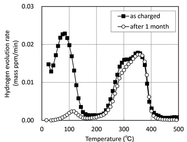
Fig. 2 Hydrogen thermal desorption analysis (TDA) curves for drawn pearlitic steel<sup>12)</sup>
