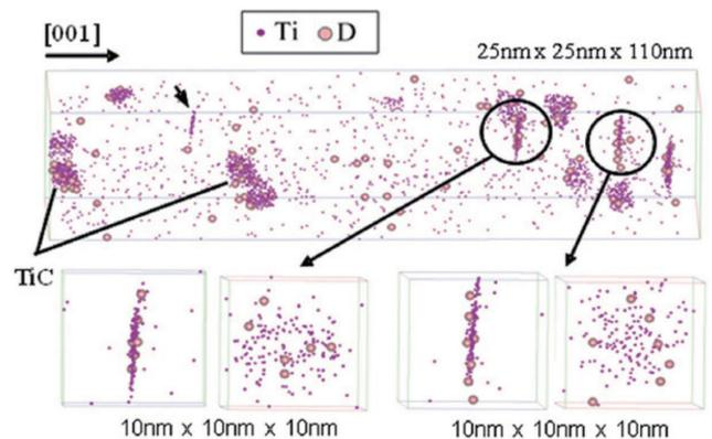
**Fig. 13** 3-dimensional mapping of deuterium-charged steel<sup>18)</sup>
