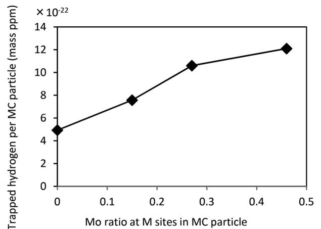
Fig. 9 Relationship between fraction of Mo in 'M' of MC and hydrogen trapping capacity per MC particle in V-Mo added 0.1%C-2.0%Mn steels<sup>15)</sup>
