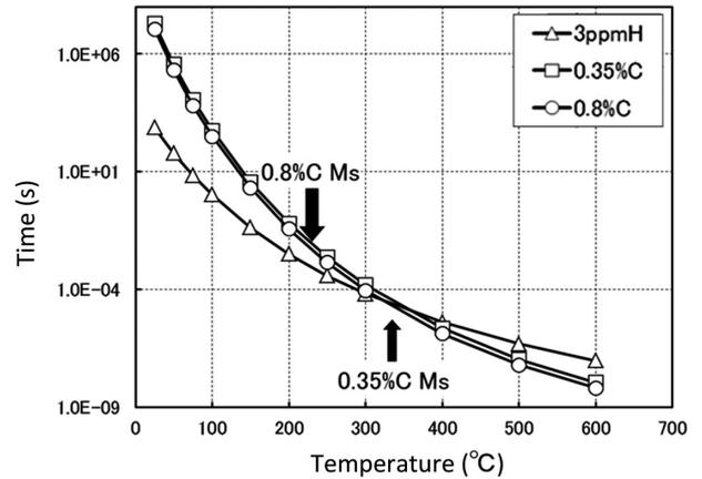
Fig. 5 Conditions for diffusion of hydrogen and carbon to reach dislocation in terms of temperature and time<sup>12</sup>
