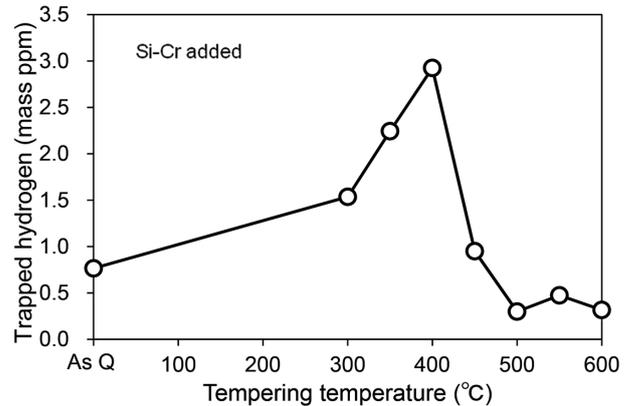
**Fig. 12** Hydrogen trapping capacity of Si-Cr added 0.6%C steels tempered at various temperatures
