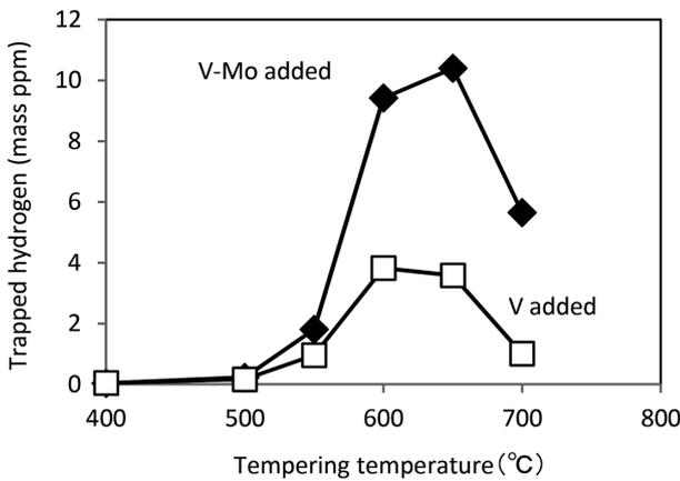
**Fig. 10** Hydrogen trapping capacity of V-Mo added 0.1%C-2.0%Mn steels tempered at various temperatures
