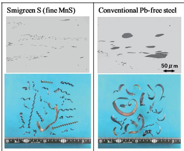
Fig. 4 Comparison of MnS morphology and chips between developed steel (SumiGreen™ S) and conventional Pb-free steel
