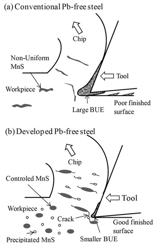
Fig. 10 Schematic illustration showing effect of MnS morphology on BUE formation
