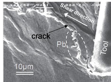
Fig. 2 Crack initiation at the primary shear zone during orthogonal cutting of leaded steel in SEM<sup>11)</sup>
