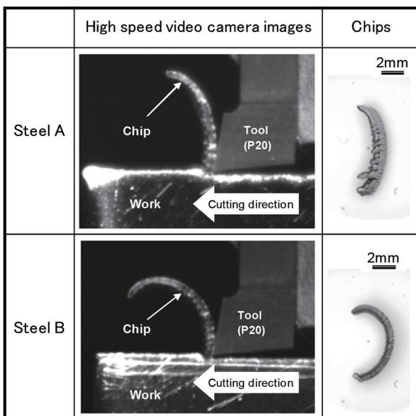
Fig. 1 In-situ observation of orthogonal cutting and chips<sup>11)</sup>
