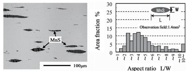
Fig. 6 MnS morphology of developed low-C free cutting steel<sup>16)</sup>
