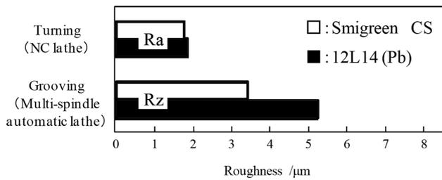
Fig. 7 Machinability in developed steel (SumiGreen™ CS)
