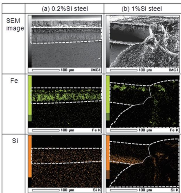
Fig. 12 SEM images of flank wear land and corresponding EDS analysis results
