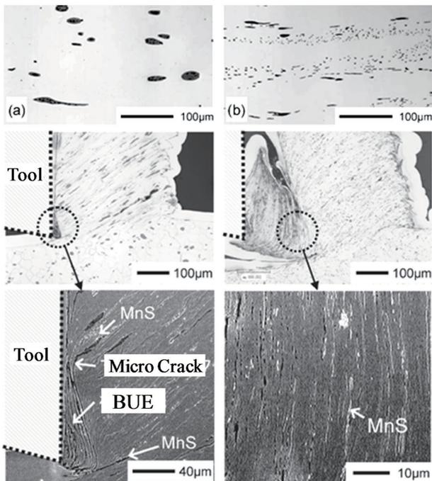
Fig. 9 Effect of MnS morphology on BUE formation<sup>16)</sup>
