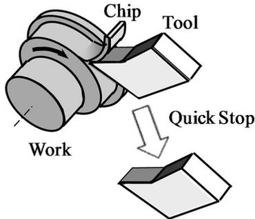
Fig. 8 Schematic illustration of quick stop test in cutting
