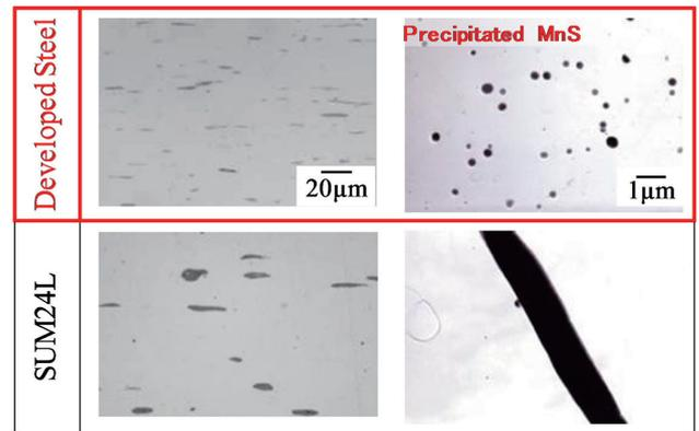
Fig. 5 Comparison of MnS morphology between developed steel and SUM24L steel
