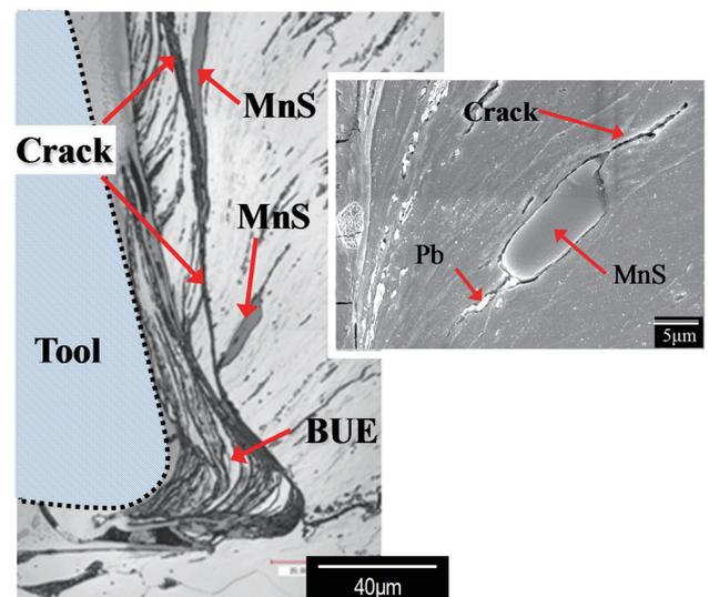
Fig. 3 Microstructure in the vicinity of built-up edge with leaded free-cutting steel, JIS SUM24L<sup>12)</sup>
