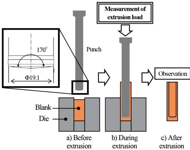
Fig. 8 Schematic drawing of evaluation method of galling resistance characteristics
