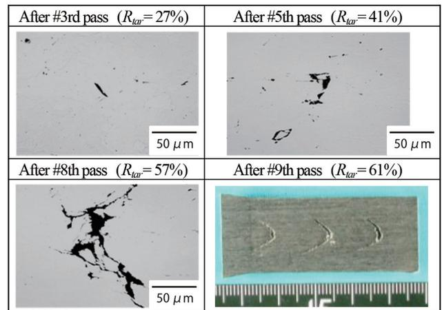
Fig. 7 Generation and growth of chevron crack
