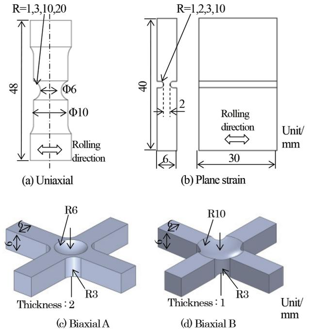
Fig. 2 Specimen for evaluation of fracture criterion
