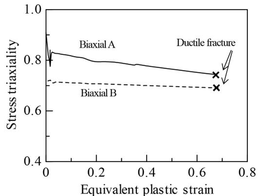
Fig. 3 Effect of specimen profile on stress triaxiality
