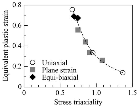
Fig. 4 Effect of multiaxial stress condition on fracture criterion in equivalent plastic strain-stress triaxiality
