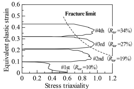
Fig. 6 Fracture prediction using fracture criterion on equivalent plastic strain-stress triaxiality
