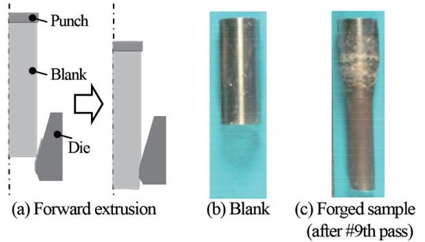
Fig. 5 Forward extrusion test
