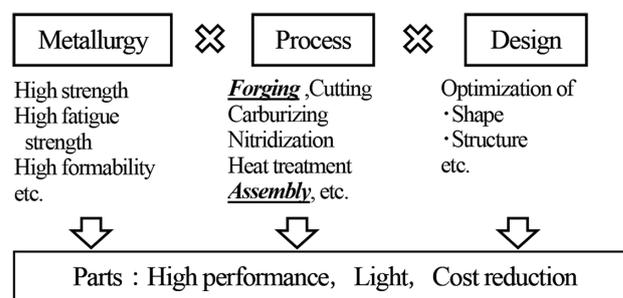
Fig. 1 Development process of high performance parts produced with steel bar and wire rod
