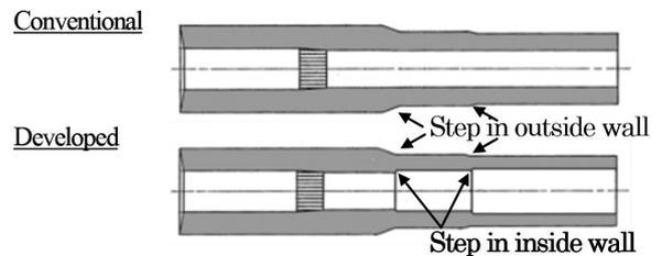
Fig. 10 Test sample of parts with long hole in the center
