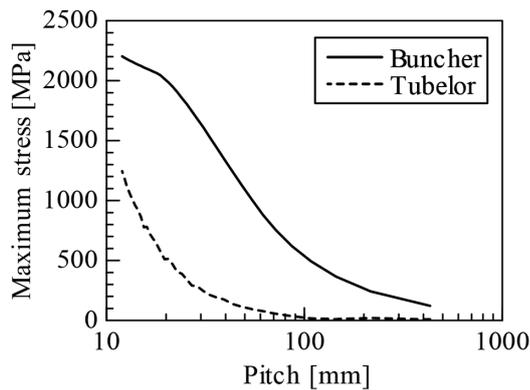
Fig. 14 Effect of strand pitch on maximum stress
