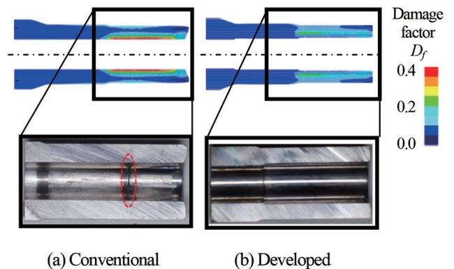
Fig. 11 Countermeasure against fracture along inside wall during forging of parts with long hole in the center
