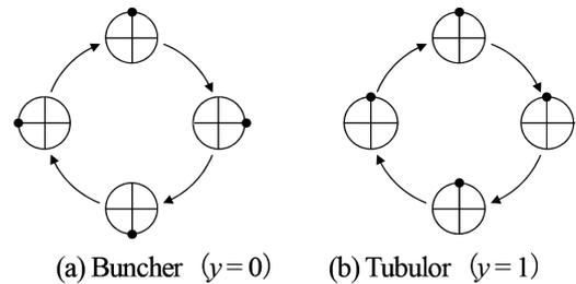
Fig. 12 Schematic view of buncher bunching and tubelor bunching
