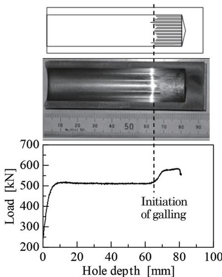
Fig. 9 Example of evaluation results of galling resistance characteristics by means of suggested method
