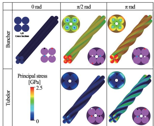
Fig. 13 Comparison of principal stress distribution between buncher bunching and tubelor bunching
