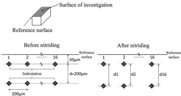
**Fig. 1 Method of measuring distortion**
