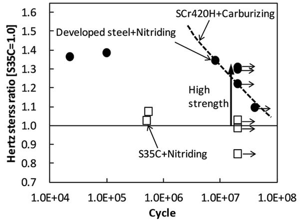
Fig. 13 Results of roller pitting fatigue test
