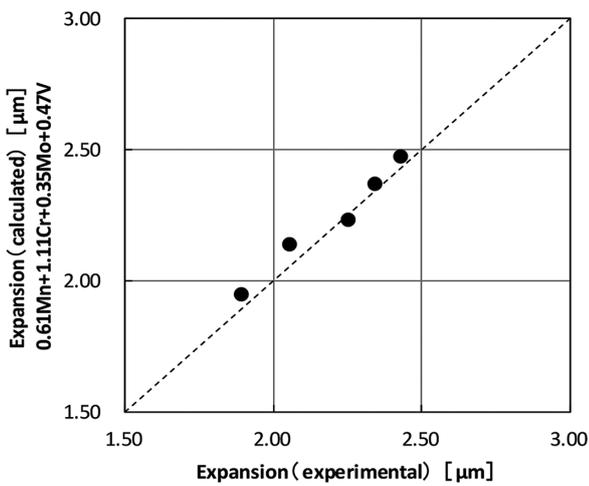
Fig. 11 Expansion due to nitriding
