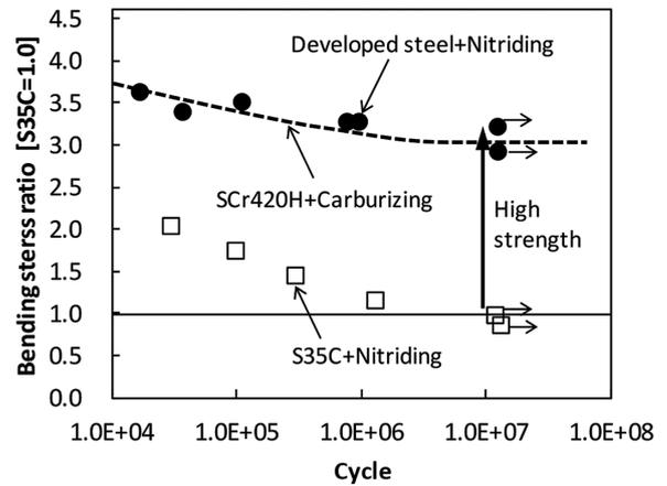
Fig. 12 Results of Ono-type bending fatigue test
