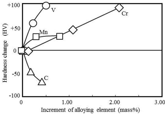
Fig. 10 Influence of alloying elements on surface hardness after nitriding
