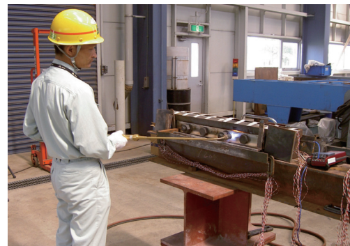
Photo 8 Heating experiment of SMA fish-plate
