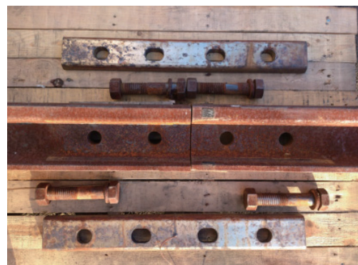
Photo 10 Dismantlement of the exposure test specimen
