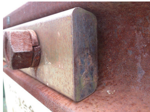
Photo 9 Exposure test of a steel fish-plate attached to a crane rail
