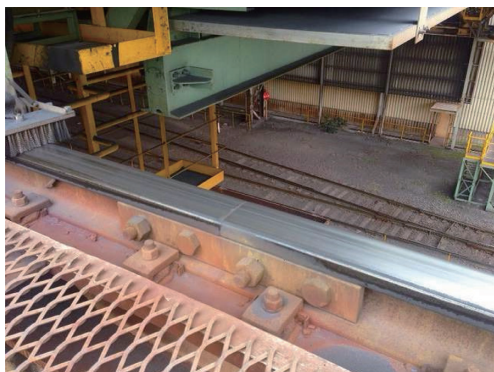
Photo 11 Installation of SMA fish-plates at the steel-making plant in Kimitsu Works
