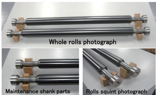
**Fig. 8** Work rolls appearance photograph after the DLC film deposition
