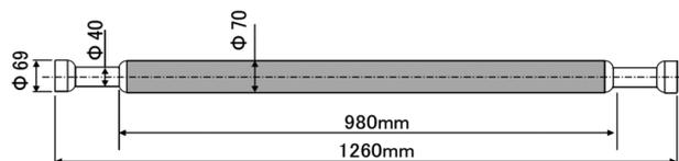
Fig. 1 Shape of the work roll for DLC film deposition
