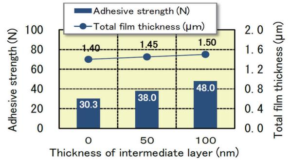
Fig. 5 Improvement effect of the adhesive strength by intermediate layer
