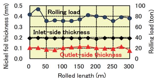
**Fig. 10** Thickness amount of change of the nickel foil in the rolling process
