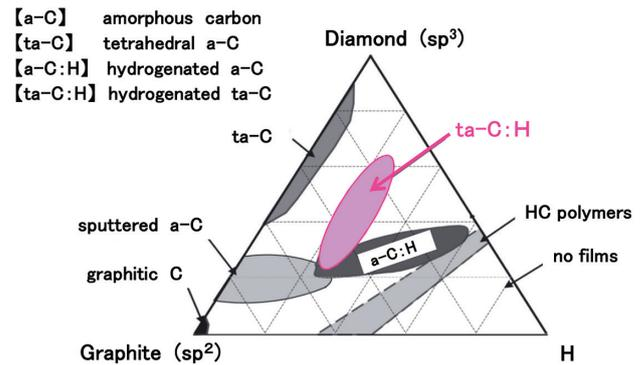
Fig. 2(a) Ternary phase diagram of amorphous carbon
