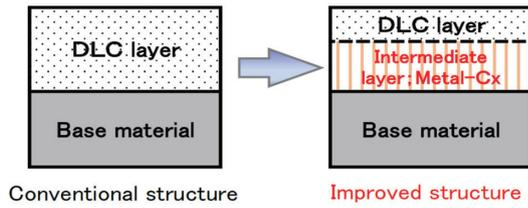
Fig. 4 Film formation structure of the work roll surface
