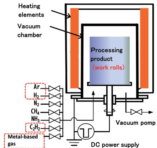
Fig. 3 CVD equipment for DLC film deposition
