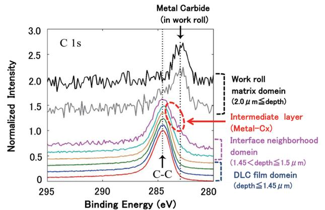
Fig. 6 Carbon 1s orbital energy analysis result of the depth direction by XPS
