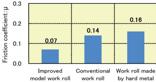
Fig. 12 Analysis results of the friction coefficient of the work rolls
