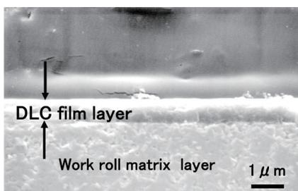
**Fig. 7** SEM microphotograph of the work roll sectional structure
