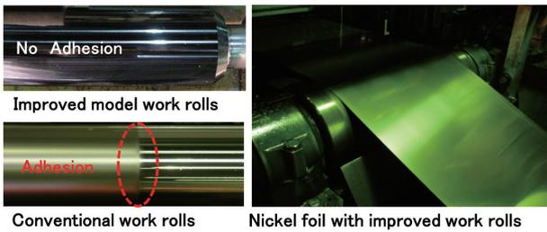
Fig. 11 Surface state of the work rolls and the nickel foil after the cold rolling examination
