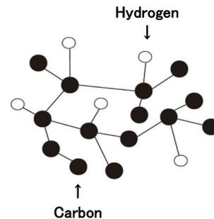
Fig. 2(b) Structure of diamond-like carbon (DLC) films (mixture of diamond structure and graphite structure)
