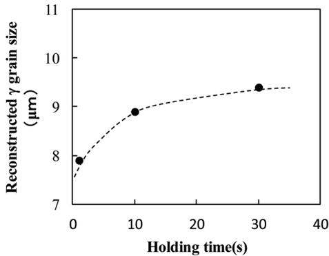
Fig. 9 Changes of grain size of reconstructed austenite microstructure to holding time at 870°C
