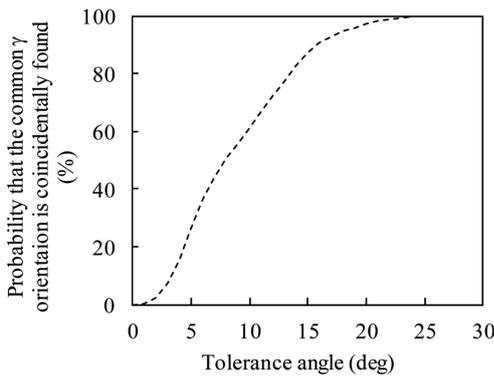
Fig. 3 Probability that a common  $\gamma$  orientation is coincidentally found between two variants for different cases of tolerance angles
