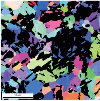
Fig. 4 Reconstructed  $\gamma$  microstructure using the variants in Fig. 1 which has just one candidating  $\gamma$  orientation
