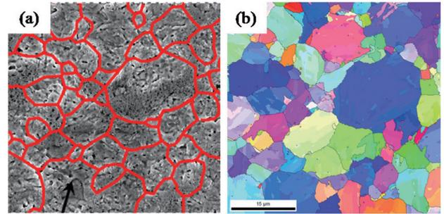
Fig. 6 Appropriateness of the grain boundaries of reconstructed austenite
