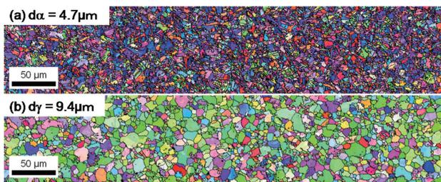
Fig. 8 Orientation mapping by EBSD analysis
