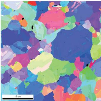
Fig. 5 Orientation mapping of  $\gamma$  microstructure reconstructed from the martensite microstructure shown in Fig. 1
