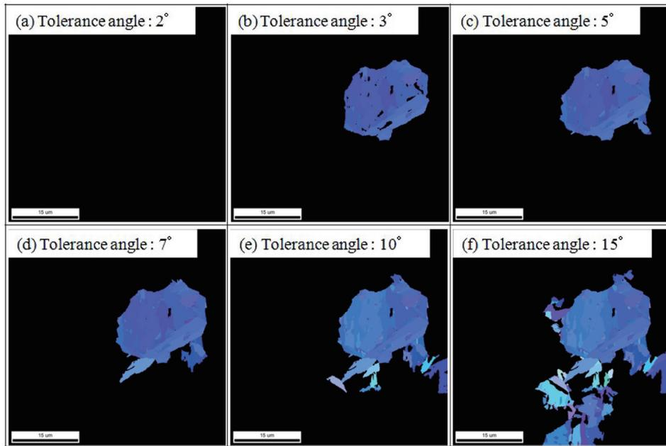
Fig. 2 Group of variants with common prior  $\gamma$  orientation for different tolerance angles (indicated as orientation mapping)
