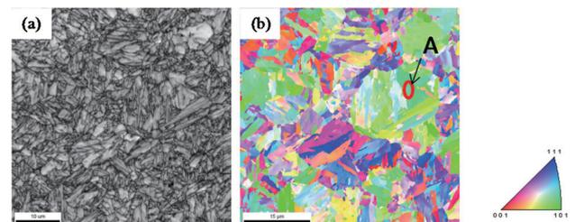
Fig. 1 Image quality mapping of the microstructure (a) and corresponding orientation mapping (b) of the specimen
