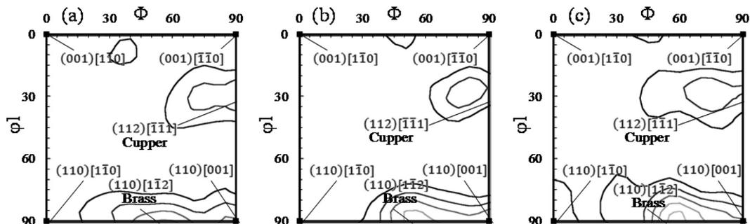
Fig. 10 Changes of the texture of reconstructed austenite microstructure to holding time ( $\phi_2=45^\circ$  section in ODF, (a) after 870°C x 1s hold, (b) after 870°C x 10s hold, (c) after 870°C x 30s hold)
