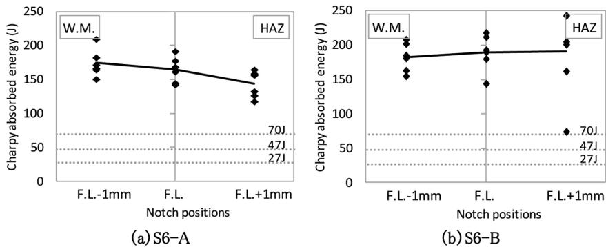
Fig. 3 Results of SAW Charpy impact test
