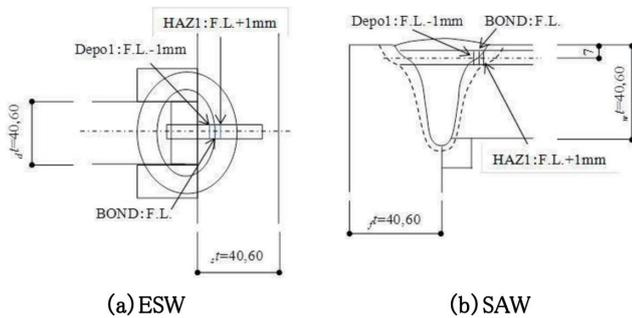
Fig. 1 Specimen and V-notch positions of Charpy impact test
