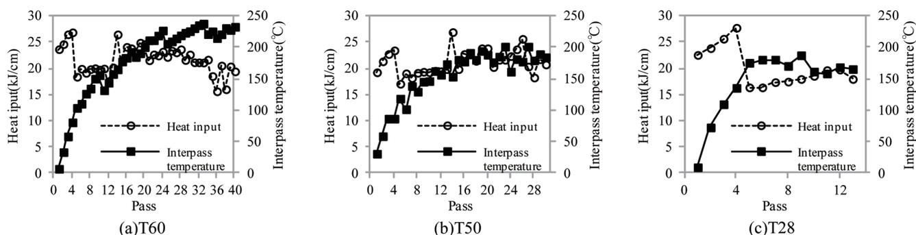
Fig. 4 Heat input and interpass temperature records
