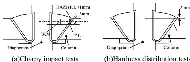
Fig. 5 Positions of specimens for Charpy impact tests and hardness distribution tests
