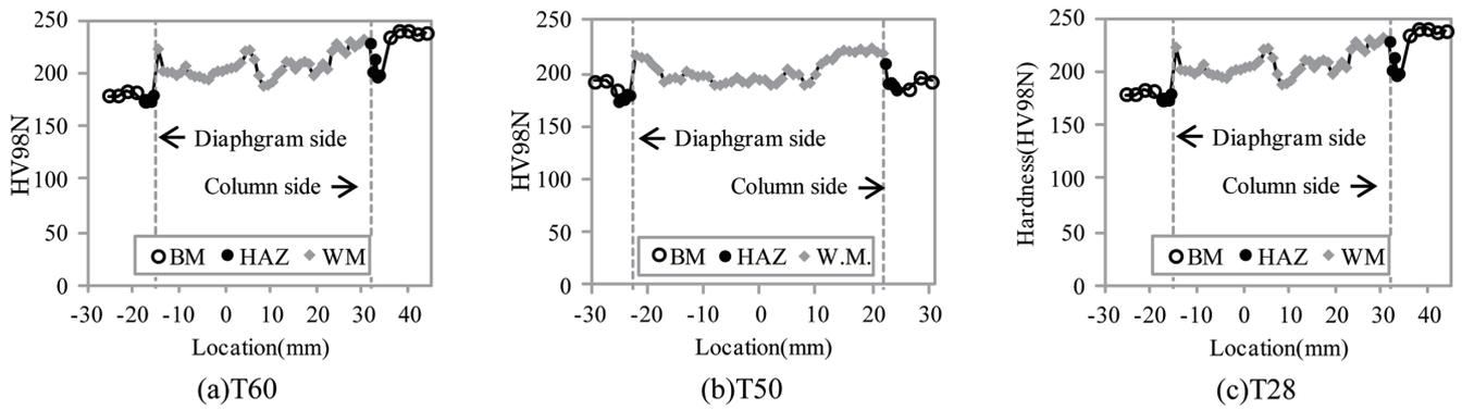
Fig. 6 Hardness distribution tests results of welded joints
