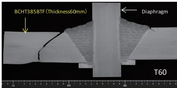
Photo 2 Macrostructure around fracture origin (thickness 60 mm)
