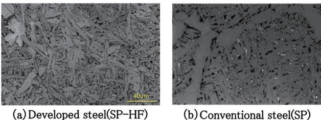
Photo 1 HAZ microstructure of ESW fusion zone
