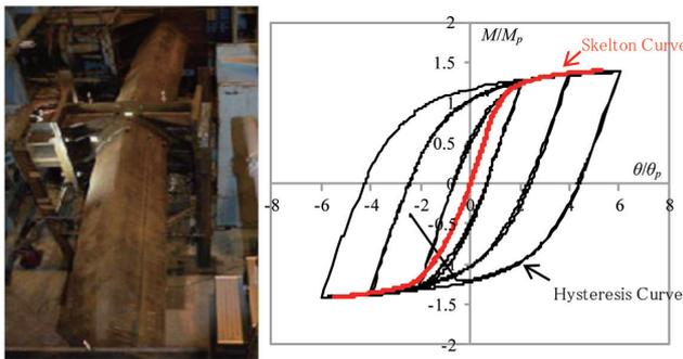
Fig. 7 Hysteretic behavior of BCHT385BTF (thickness 60 mm)
