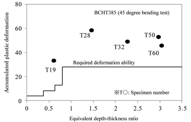
Fig. 8 Effect of depth-thickness ratio on accumulated plastic deformation (BCHT385BTF)
