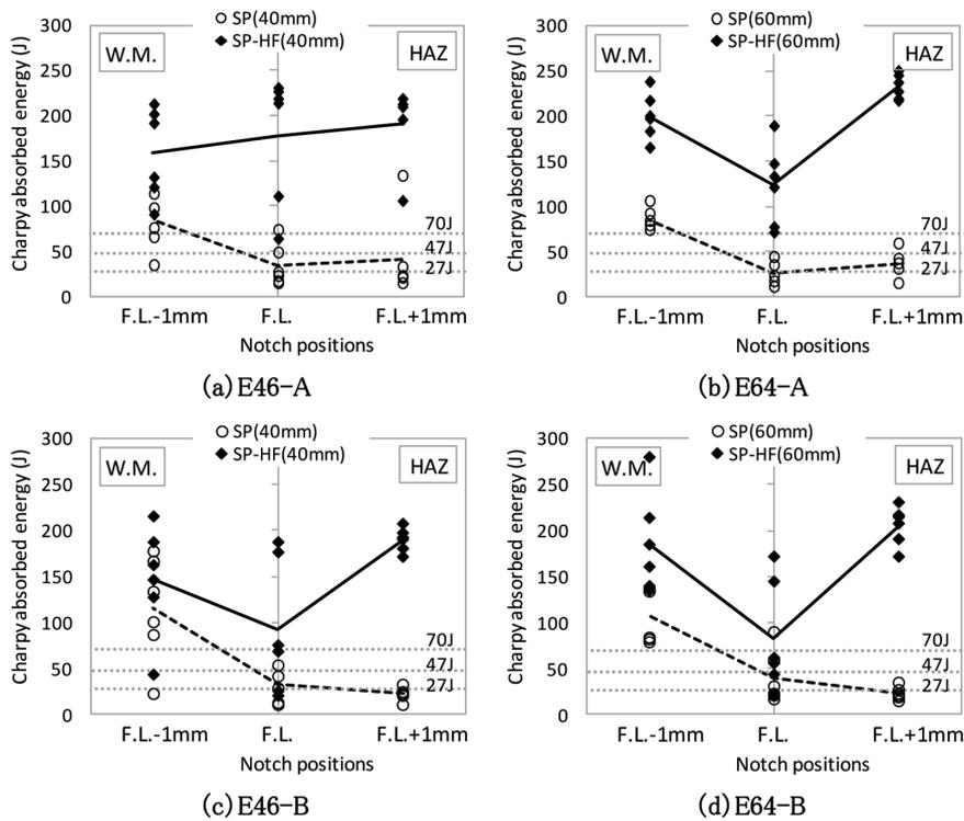
Fig. 2 Results of ESW Charpy impact test
