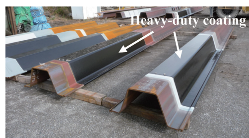
Photo 7 Hat-shaped sheet pile protected by heavy-duty coating
