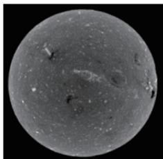
Photo 4 X-ray-CT result of the core
