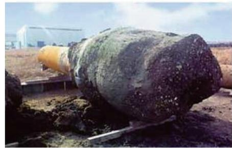
Photo 2 Photo of turned pile (D: 1000 mm)
