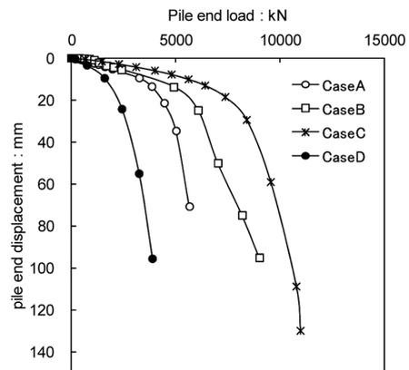
Fig. 10 Pile end load and pile end displacement
