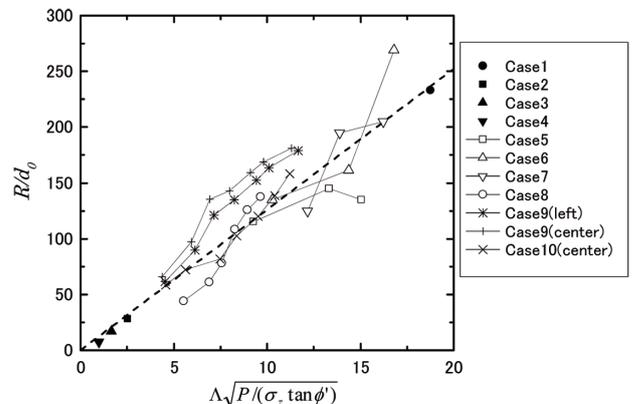
Fig. 6 Relationship among the WJ specification, soil resistance and jet penetration distance
