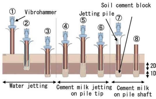
Fig. 1 Construction process
