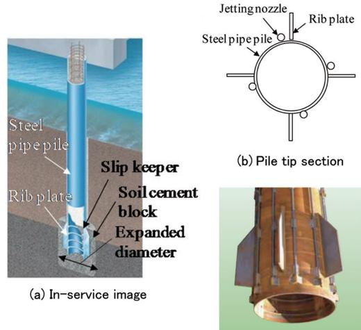
Fig. 3 Outer rib plate type
