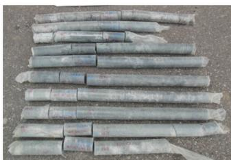
Photo 3 Soil-cement core bored from pile
