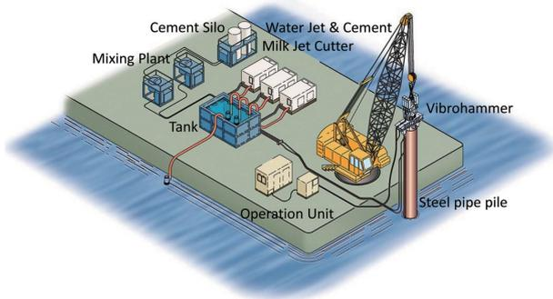
Fig. 2 Construction facilities
