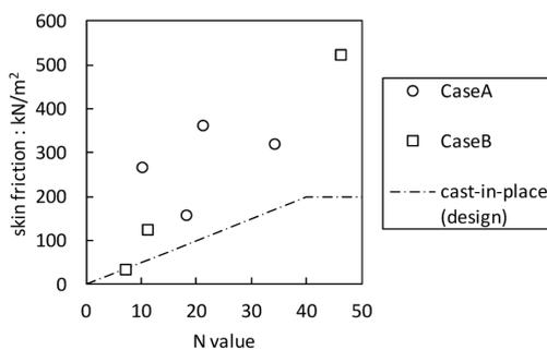
Fig. 11 Relationship between SPT-N and skin friction on sand
