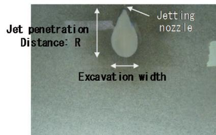
Photo 1 Sample of the centrifuge jetting experiment
