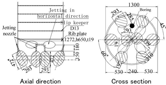
Fig. 9 Position of jetting nozzle and supposed excavation area
