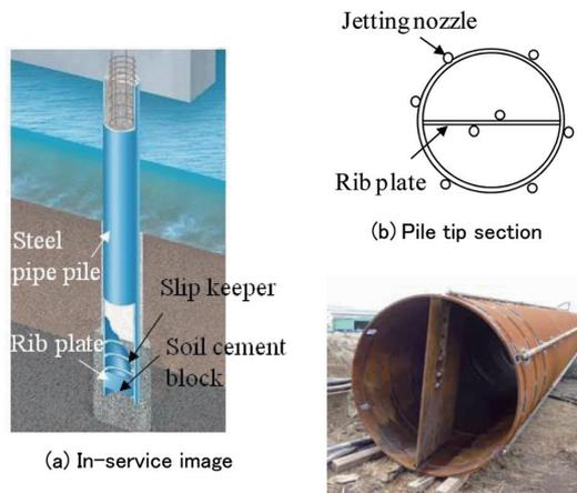
Fig. 4 Inner rib plate type
