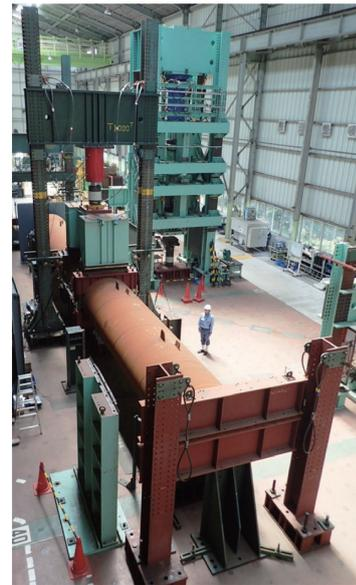
Photo 2 Photo of bending test ( $\phi 1600 \times t19 \text{ mm}$ )
