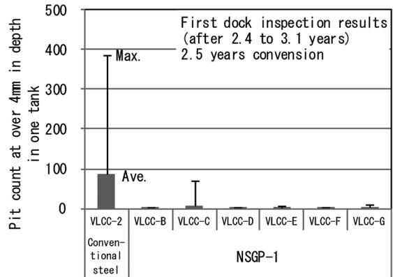
Fig. 5 Observed pit count of VLCC-2 using conventional steel and six VLCCs using NSGP-1
