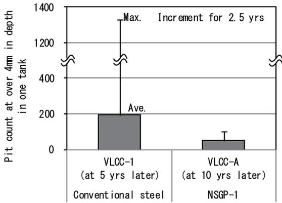
Fig. 3 Observed pit count for VLCC-1 using conventional steel upon 5-year and VLCC-A using NSGP-1 upon 10-year inspection
