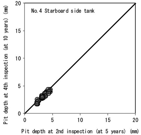
Fig. 4 Depth measurement result of the fifth year and the tenth year of the same pits
