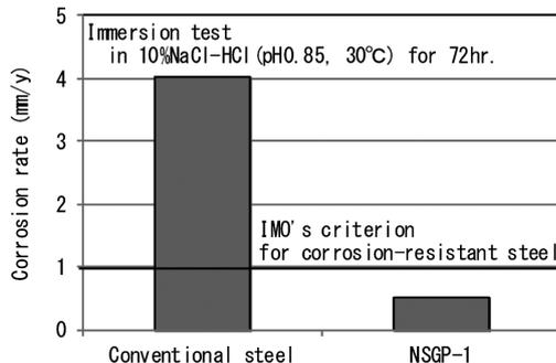
Fig. 2 Corrosion test results of NSGP-1 and conventional steel
