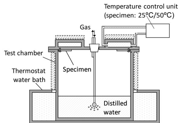
**Fig. 7 Simulated corrosion test apparatus for upper deck of COT**
