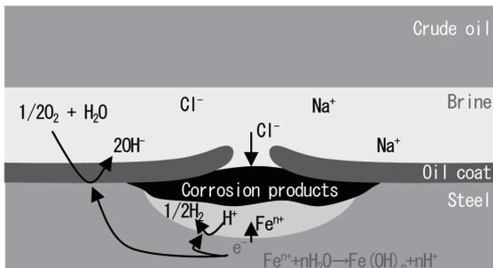
Fig. 1 Summarized process and mechanism of localized corrosion on COT bottom plate
