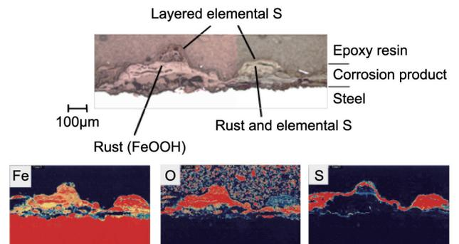
**Fig. 8 Cross sectional morphology and distribution of elements by electron probe micro analyzer (EPMA) in corrosion product of specimen after simulated corrosion test for upper deck**
