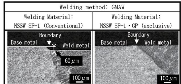
Photo 1 Cross section view of welded joints of NSGP-1 after corrosion test
