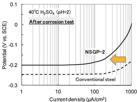
**Fig. 9** Anodic polarization curves of conventional steel and NSGP-2
