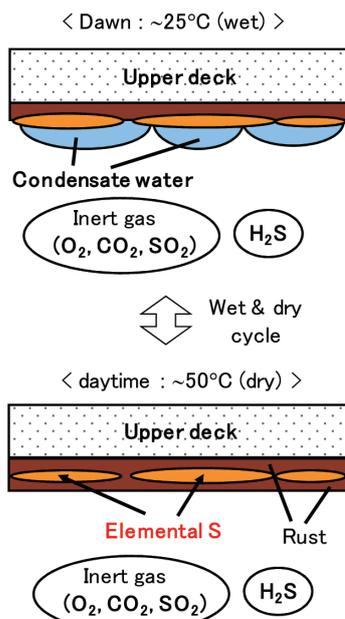
**Fig. 6 Corrosion mechanism at COT upper deck plate**
