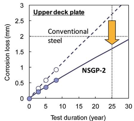
**Fig. 10** Onboard test results of NSGP-2 and estimated corrosion loss after 25 years
