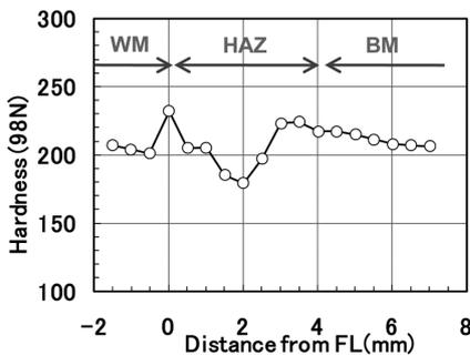
Fig. 12 Hardness distribution of welded joint (25 mm)
