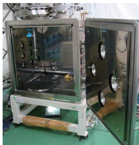
Fig. 15 Precision machinery (vacuum vessel) of ARU-TEN
