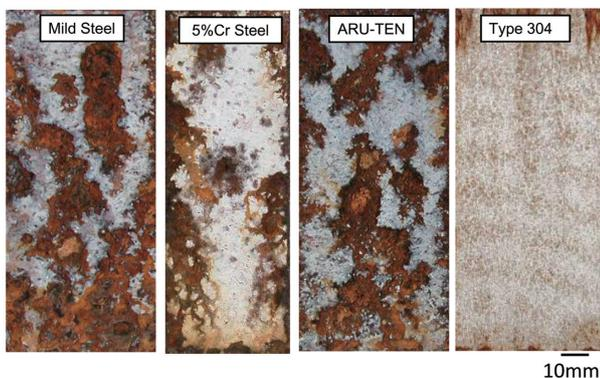
**Fig. 1** Appearance of samples (bare surface) after corrosion test for 90 cycles<sup>9)</sup>
