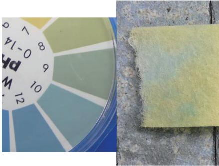
Fig. 4 Measurement result of pH on Zn-primer painted corrosion product after CCT
