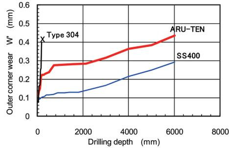
Fig. 13 Influence of materials on outer corner wear of drill tip
