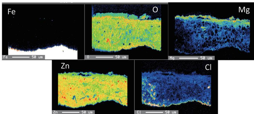
Fig. 8 EPMA analysis results of cross-section of rust layer on Zn-primer painted steel for after CCT
