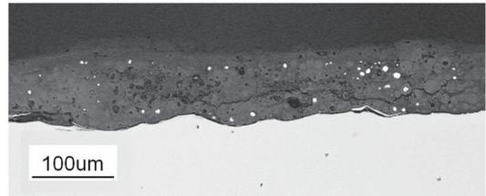
Fig. 7 Optical microphotographs of cross-section of rust layer on Zn-primer painted samples after CCT
