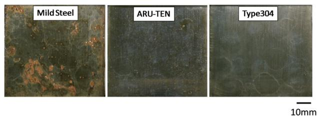
Fig. 9 Appearance of samples (bare surface) after condensation corrosion test for 300 h
