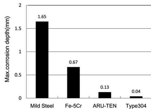
**Fig. 3** Maximum corrosion depth of samples after corrosion test for 150 cycles<sup>9)</sup>
