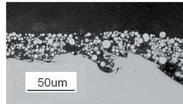
Fig. 6 Example of optical microphotographs of cross-section of Zn-primer painted samples (before test) (zinc content of heating residue: about 80%, aimed coating thickness 25 μm)
