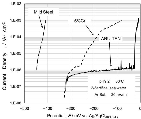
Fig. 5 Anodic polarization curves of mild steel, 5%Cr and ARU-TEN in mixed solution of artificial sea water and standard buffer solution, with its pH 9.2
