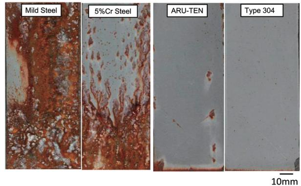
**Fig. 2** Appearance of Zn-primer painted samples after corrosion test for 150 cycles<sup>9)</sup>
