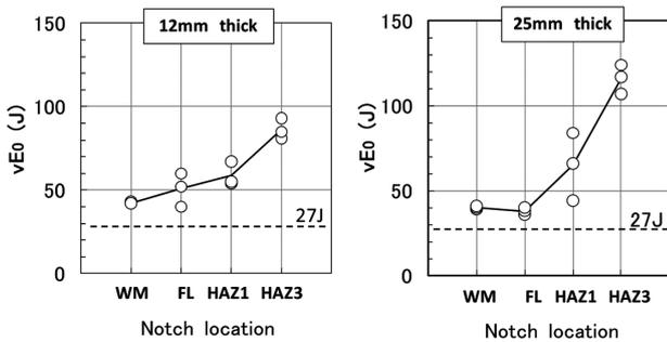
Fig. 11 Test results of Charpy impact test
