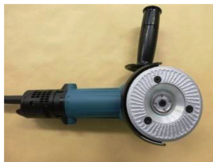
Fig. 16 Grinder with manmade diamond grains
