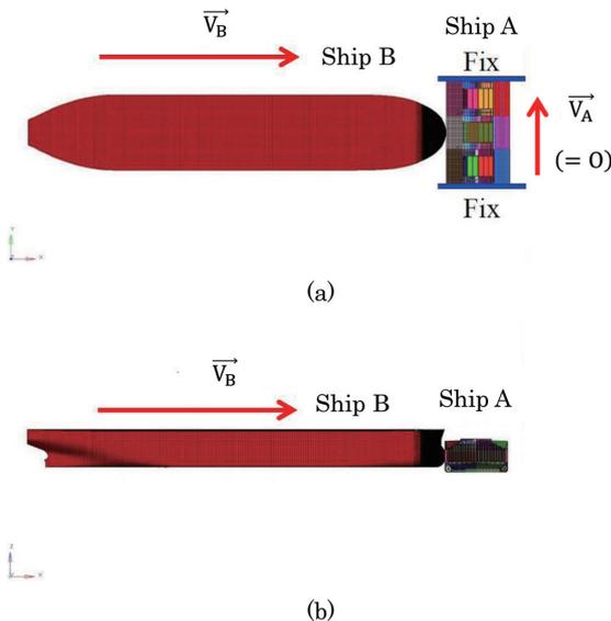
Fig. 5 Side-collision model for bulk carrier (courtesy of National Maritime Research Institute) (a) Plan view, (b) Front view
