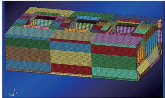
Fig. 6 FEM model of struck ship used (courtesy of National Maritime Research Institute)
