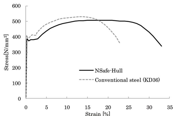
**Fig. 1** Examples of stress-strain curves
