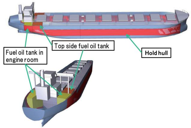
Fig. 3 Overview of parts for which NSafe-Hull is world-first used (courtesy of Imabari Shipbuilding Co., Ltd.)
