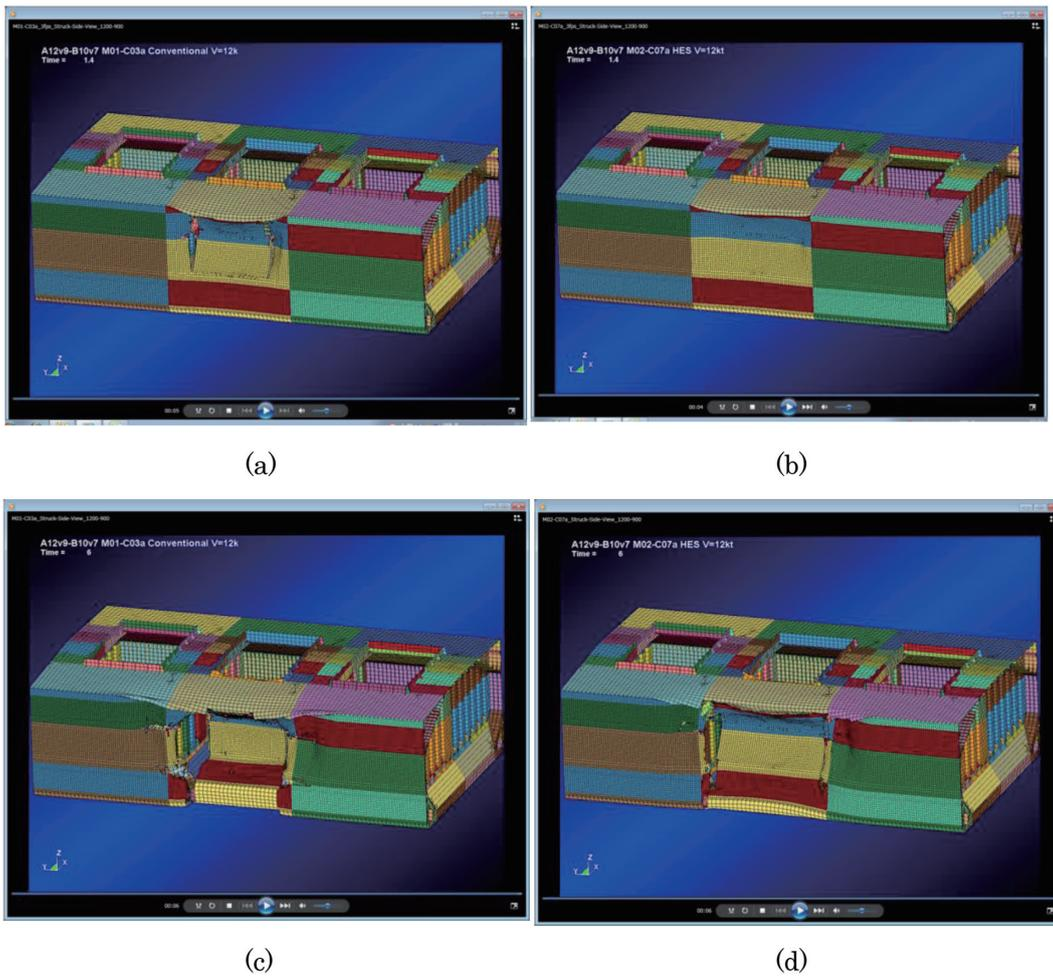
Fig. 8 Comparisons of damage in struck (at 12 knots) ship with conventional steel and NSafe-Hull in hull structure (a) 1.4 seconds after collision with conventional steel, (b) 1.4 seconds after collision with NSafe-Hull, (c) 6 seconds after collision with conventional steel, (d) 6 seconds after collision with NSafe-Hull
