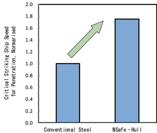
Fig. 10 Critical striking ship speed for penetration, normalised by value of case with conventional steel
