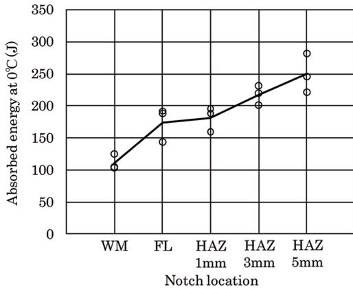
Fig. 2 Charpy impact test results of welded joint
