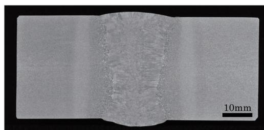
**Photo 1** Macrostructure of welded joint
