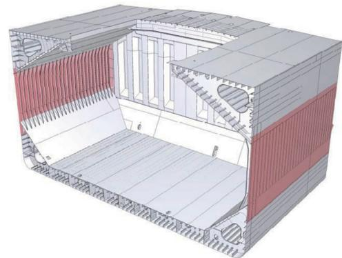
Fig. 7 Sectioned view of parts for which NSafe-Hull is used (parts in red)
