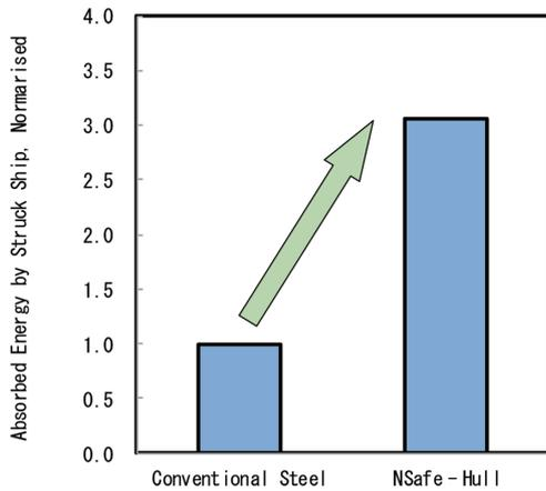
Fig. 9 Absorbed energy by struck ship, normalised by value of case with conventional steel
