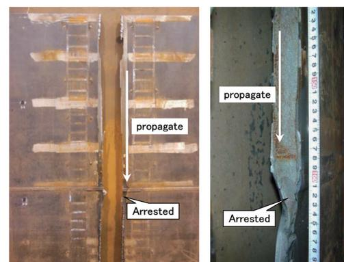
Fig. 7 Example of large scale fracture test
