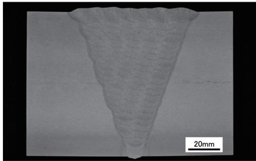
Fig. 8 Macrostructure of welded joint
