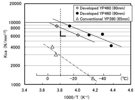
Fig. 5 Results of temperature gradient type ESSO test
