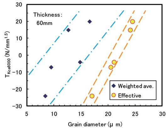
Fig. 3 Relationship between grain diameter estimated by EBSD and  $T_{Kca6000}$  obtained by ESSO test
