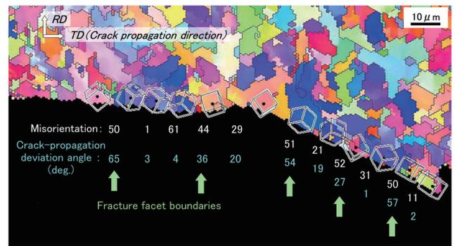
Fig. 2 Example of analysis to estimate effective grain size by EBSD
