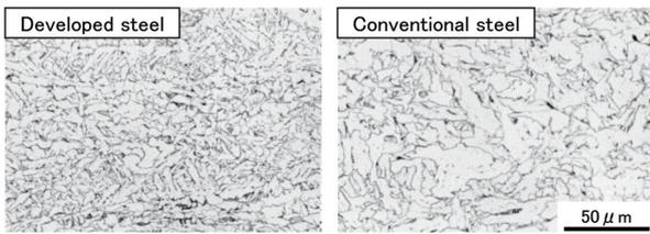
Fig. 4 Microstructures of developed steel and conventional steel
