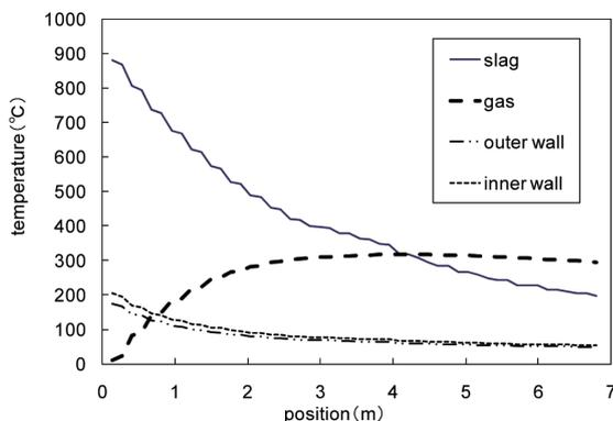
Fig. 6 Temperature simulation with internal water spray
