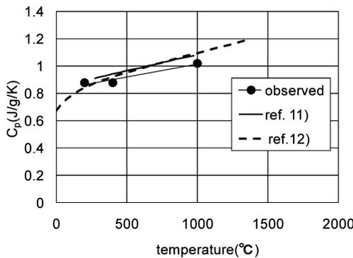
**Fig. 1** Temperature dependence of the slag specific heat
