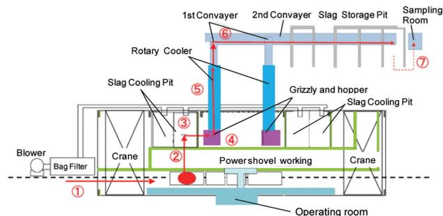
Fig. 7 Layout of the ORP slag processing plant
