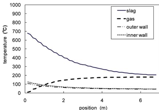
Fig. 5 Temperature simulation without internal water spray
