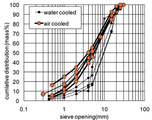
**Fig. 2** Particle size distribution (cumulative) of slag
