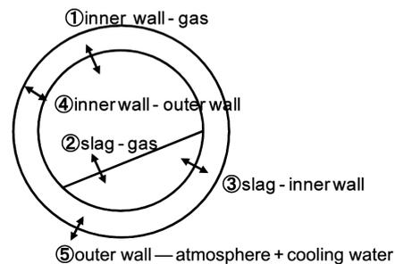
**Fig. 3** Concept diagram of the heat transfer mechanism
