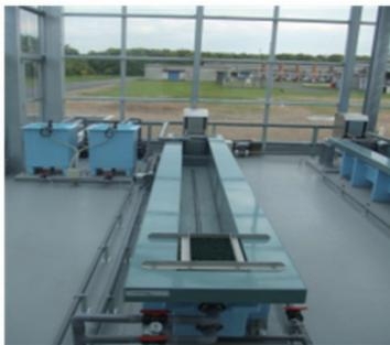
Fig. 8 Experimental apparatus for shallow seabed<sup>3)</sup>
