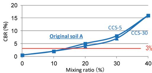
**Fig. 10 Relationship between CBR and mixing ratio**
