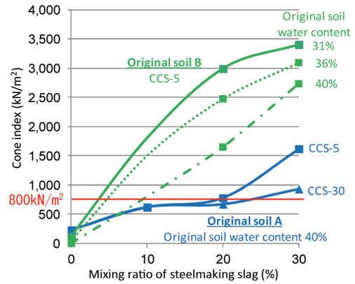
Fig. 8 Relationship between cone index and mixing ratio of steelmaking slag
