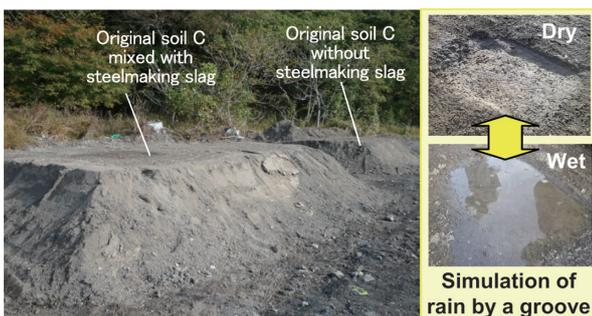
**Fig. 11 Result of test banking**
