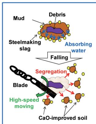
Fig. 3 Image of absorbing water effect
