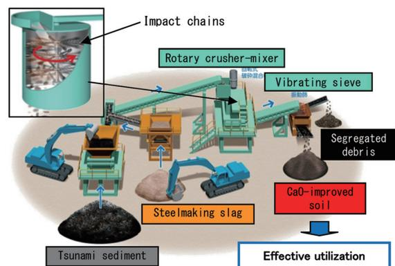
Fig. 1 High-speed rotary CaO-improvement method
