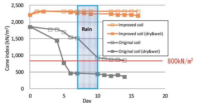
**Fig. 12 Changes of cone index under drying and wetting**
