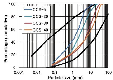
Fig. 7 Particle size distribution of steelmaking slag
