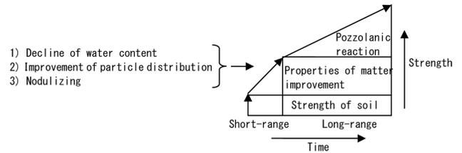
Fig. 5 Schematic illustration of lime strengthening (quoted from a literature of Japan Cement Association)
