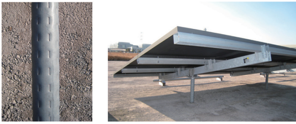
Fig. 23 Pipe with surface dimples (left), and application example as foundation pilings for solar panels (right)
