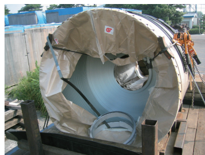
Photo 1 Coil collapse accident example
