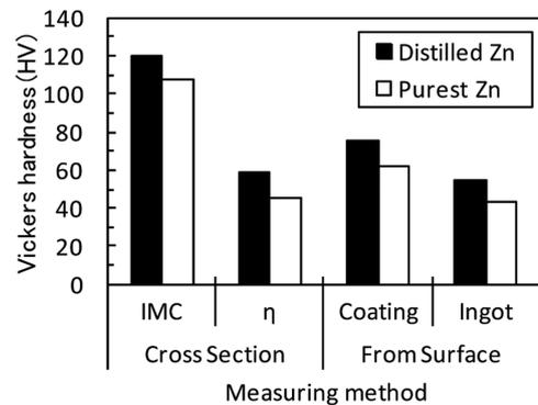
Fig. 8 Vickers hardness of coating
