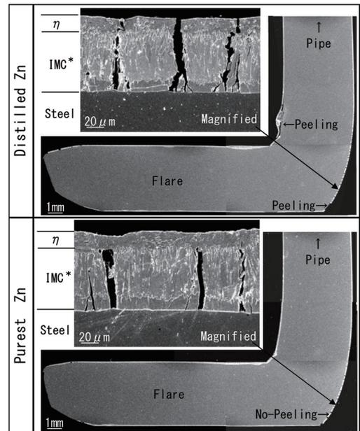
Fig. 7 SEM (scanning electron microscope) image on the cross section of flared coating
