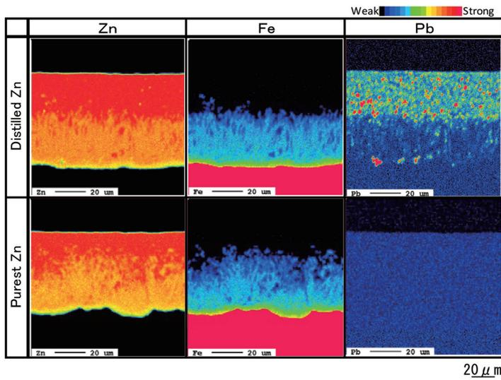
Fig. 4 EPMA element mapping on cross section of coating
