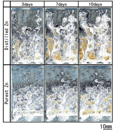
Fig. 5 Views after SST corrosion test
