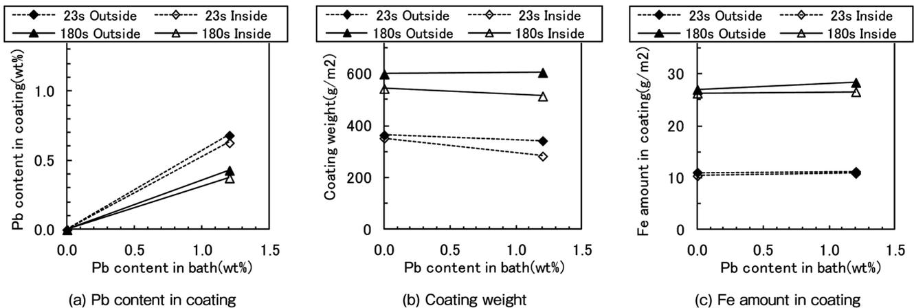
Fig. 2 Chemical analysis of coating (seconds are dipping time in bath)
