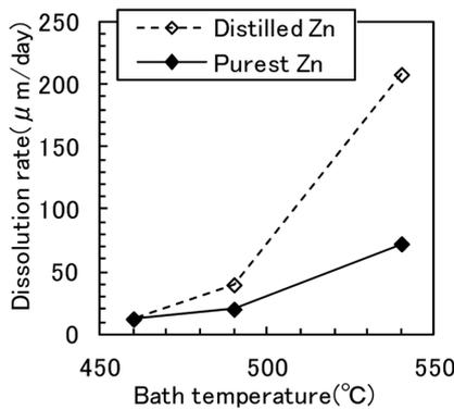
Fig. 10 Dissolution rate of bath steel
