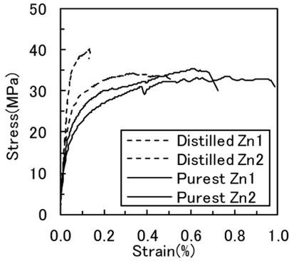
Fig. 9 Tensile test of Zn
