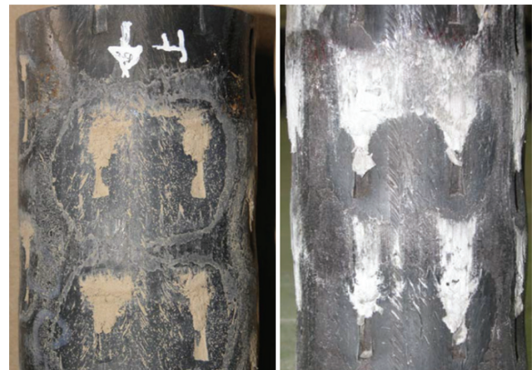
Fig. 13 Outer surfaces of pipes after bonding test (left: soil-cement of 2 MPa; right: mortar of 36 MPa)
