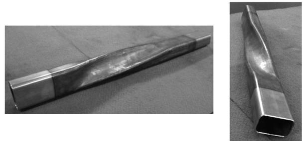
Fig. 12 Example of twisting by 3DQ
