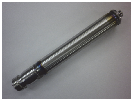
Fig. 6 Curtain airbag inflator
