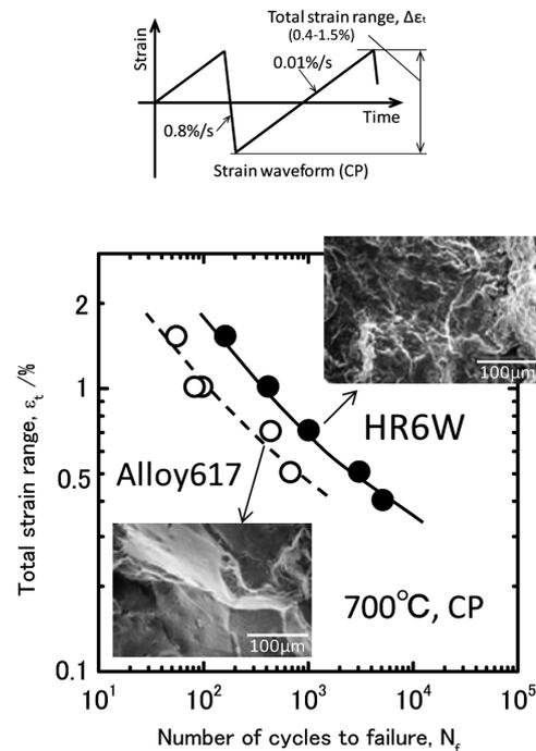
Fig. 3 Creep-fatigue properties of HR6W and Alloy 617<sup>13)</sup>
