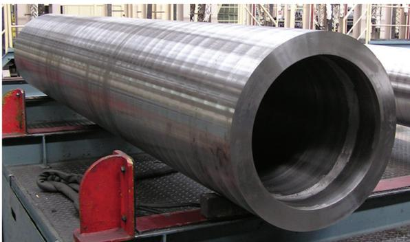
Photo 4 Appearance of HR6W thick-wall pipe
