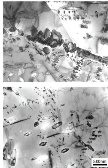
Photo 7 TEM microstructures of HR35 after creep rupture (700°C, 157 MPa, 13,110 h)
