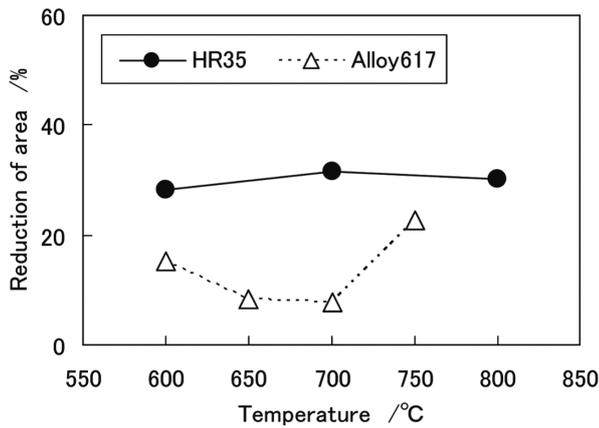
Fig. 9 Rupture ductility by extra low strain-rate tensile tests
