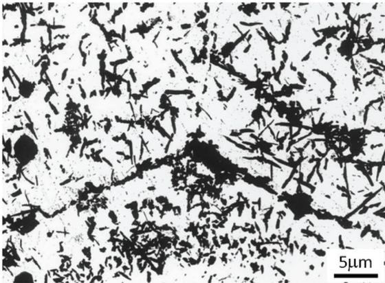
Photo 3 TEM microstructure of extracted replica of HR6W after creep rupture (700°C, 98 MPa, 58,798 h)
