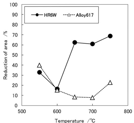
Fig. 4 Rupture ductility by extra low strain-rate tensile tests<sup>16)</sup>
