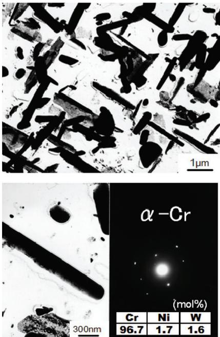
Photo 5 TEM microstructures of extracted replica of HR35 after creep rupture (750°C, 127 MPa, 2,527 h)
