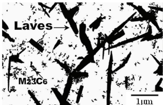
Photo 1 TEM microstructure of extracted replica of HR6W aged at 750°C for 3,000 h
