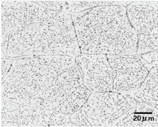
Photo 2 Optical microstructure of HR6W after creep rupture (700°C, 98 MPa, 58,798 h)
