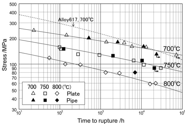
Fig. 7 Creep rupture strength of HR35
