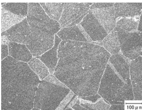
Photo 6 Optical microstructure of HR35 after creep rupture (700°C, 157 MPa, 13,110 h)
