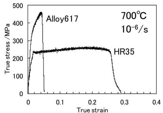
Fig. 8 S-S curves obtained by extra low strain-rate tensile tests
