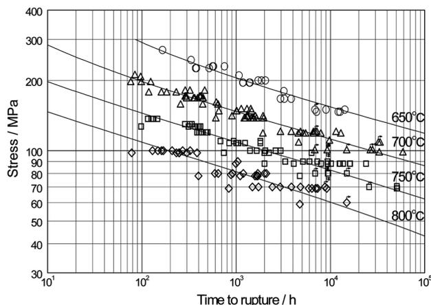
Fig. 2 Creep rupture strength of HR6W
