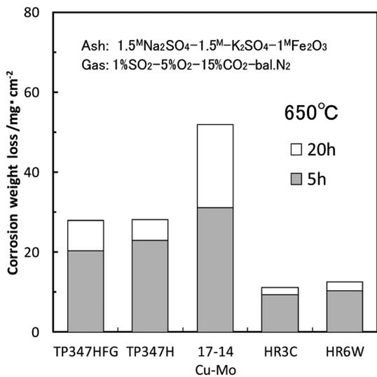
Fig. 5 High temperature corrosion properties of HR6W and other austenitic steels
