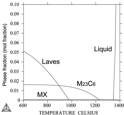
Fig. 1 Phase fractions of HR6W computed by Thermo-Calc
