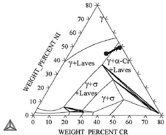
Fig. 6 Calculated phase diagram of Cr-Ni-Fe-7W system (750°C)
