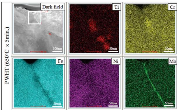
Fig. 5 Elemental distribution in the vicinity of surface at HAZ of PWHT material by STEM/EDS mapping
