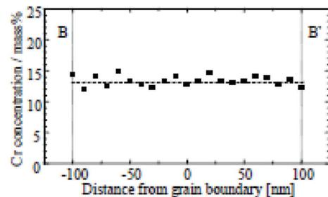
**Fig. 4** TEM micrograph at the vicinity of surface oxide layer and results of line analysis around the grain boundary by EDS for PWHT material
