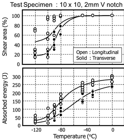
Fig. 9 Toughness of developed material
