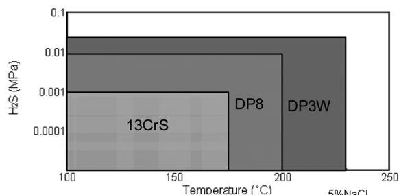
**Fig. 2** Material selection guidelines for environments
