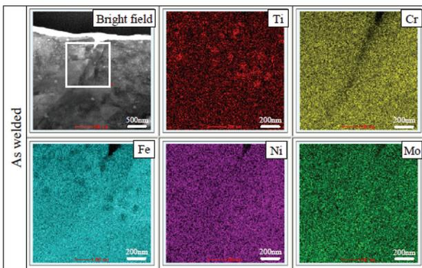
Fig. 6 Elemental distribution in the vicinity of surface at HAZ of as welded material by STEM (scanning transmission electron microscopy)/EDS mapping
