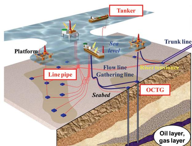
Fig. 1 Diagram of production and transportation for oil and natural gas
