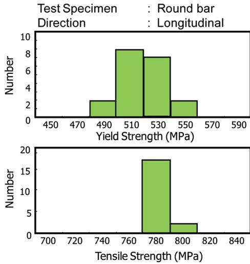
Fig. 8 Distribution for mechanical properties of developed material
