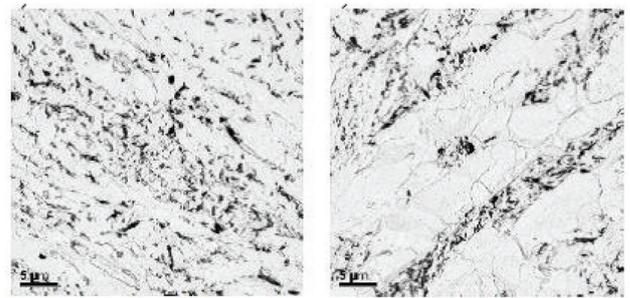
Fig. 12 TEM images of Mo-free and Mo-containing steels (left and right, respectively, in replicas)<sup>6,8)</sup>
