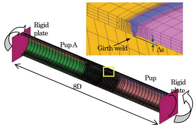
Fig. 3 Bending model for girth-welded pipe
