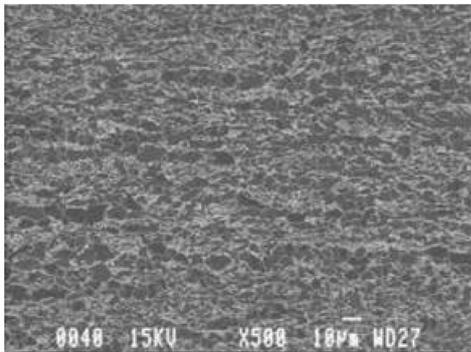
Fig. 14 SEM image showing microstructure of highly deformable pipe<sup>6, 11)</sup>
