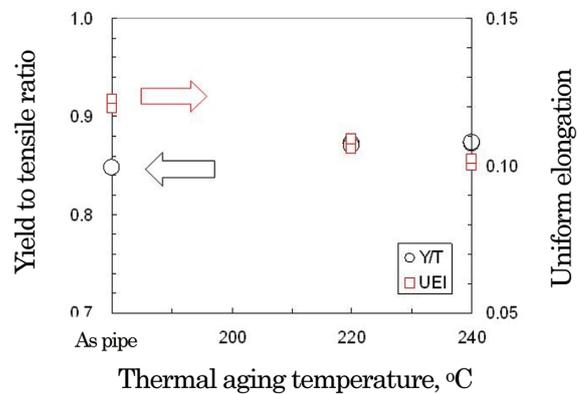
Fig. 16 Mechanical properties before and after thermal aging of API grade X60 highly deformable pipe<sup>6, 11)</sup>
