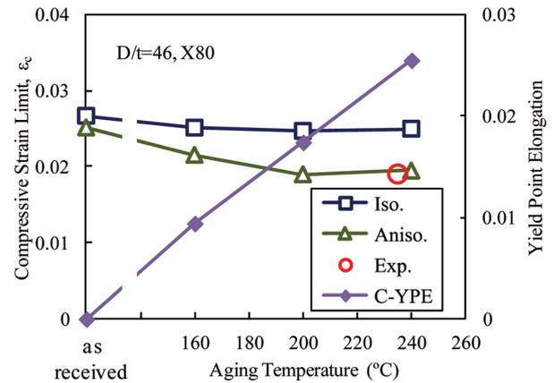
Fig. 8 Effect of C-YPE on compressive strain limit
