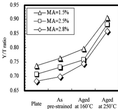
Fig. 15 Effect of M-A content on yield to tensile ratio<sup>12)</sup>
