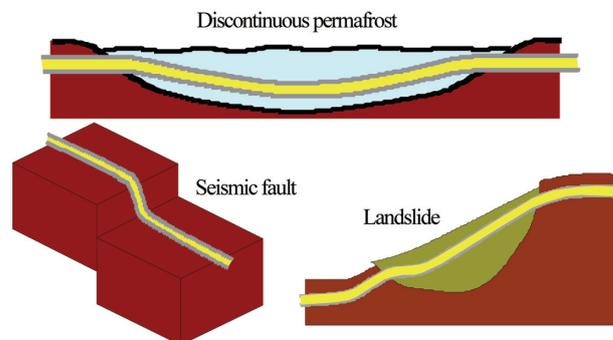
Fig. 1 Pipe deformation with ground movement
