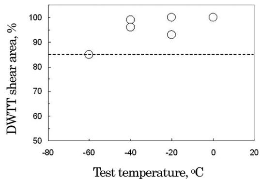
Fig. 17 DWTT properties of API grade X60 highly deformable pipe<sup>6, 11)</sup>
