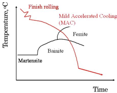
Fig. 13 Cooling curve during accelerated cooling<sup>6, 7)</sup>
