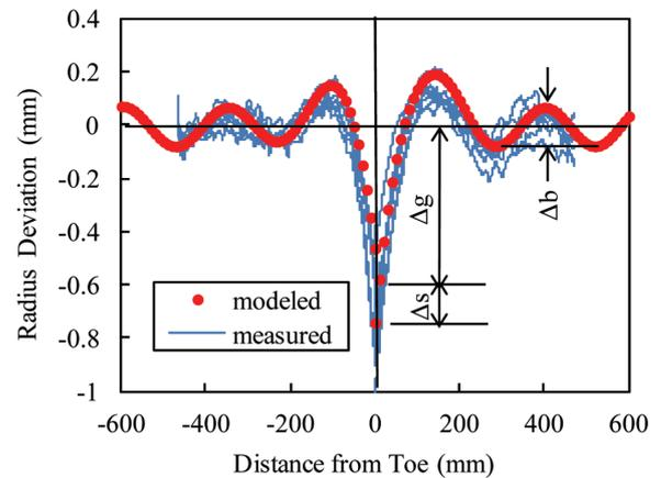
Fig. 2 Radius change in girth-welded UOE pipe
