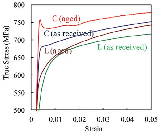
Fig. 4 Plastic anisotropy in UOE pipe
