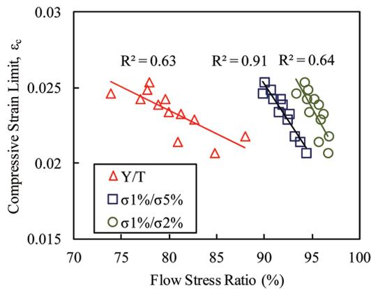
Fig. 7 Correlation between compressive strain limit and mechanical property factors
