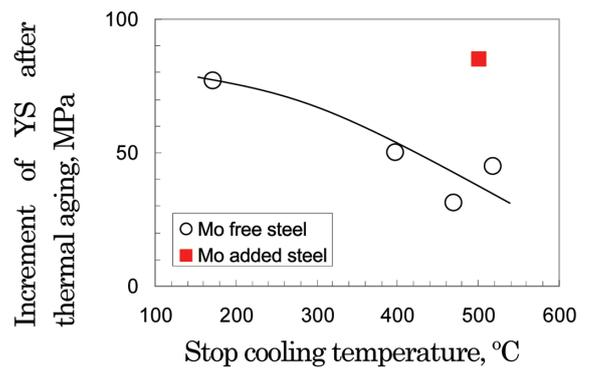
Fig. 11 Increase in YS of Mo-free and Mo-containing steels after application of 1% pre-strain and aging at  $240^\circ\text{C}$ .<sup>6,7)</sup>
