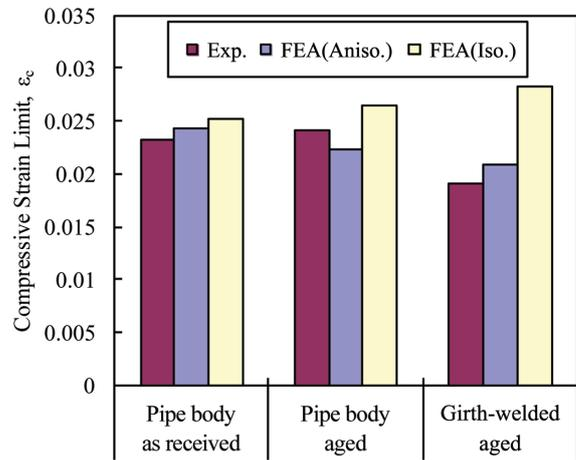
Fig. 6 Comparison of measured and calculated compressive strain limits
