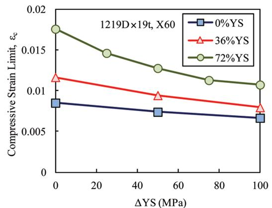
Fig. 9 Effect of strength mismatch on compressive strain limit
