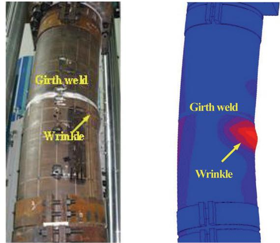
Fig. 5 Buckling behavior of girth-welded pipe under bending and plastic strain distribution
