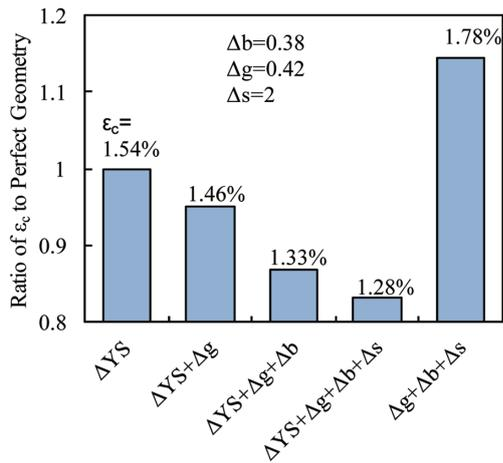
Fig. 10 Combined effect of geometric imperfection and strength mismatch on compressive strain limit
