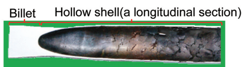
Fig. 5 Example of defect on internal surface
