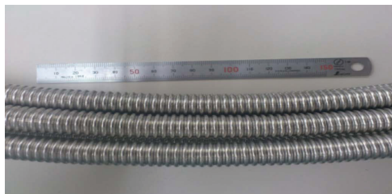
Fig. 4 Flexible tube of NSSMC-NAR-DP-3W (0.2 mm thickness × 20 mm diameter)
