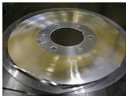
Fig. 5 Pure nickel lead for lithium-ion rechargeable battery
