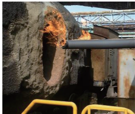
Photo 2 Burner for torpedo car used for 2 years
