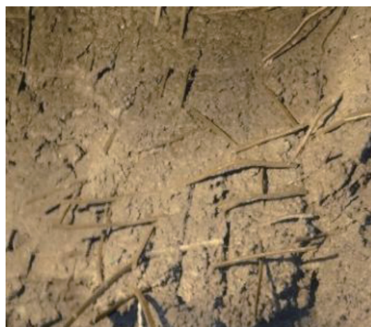
Photo 4 Inside of the gasified melting furnace after working for 2 months
