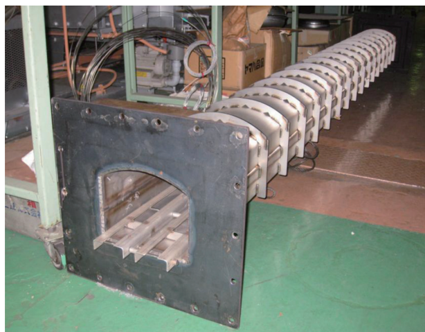
Photo 3 Example of industrial furnace application (muffle furnace Kanto Yakin Kogyo Co., LTD.)
