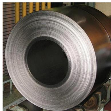
**Photo 2** Hot strip product of Super-TIX™51AF manufactured at a production mill
