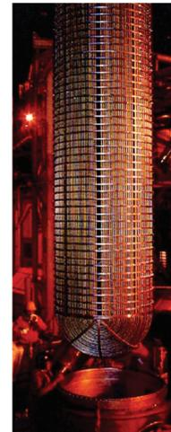
Photo 2 Oil gas coolers made of SMIACE™
