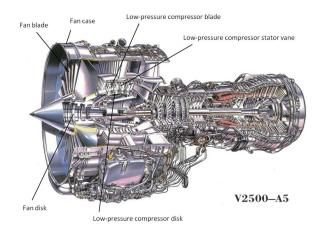
Fig. 4 Example of the application of titanium alloy for aero engine (by courtesy of Japanese Aero Engines Corporation)
