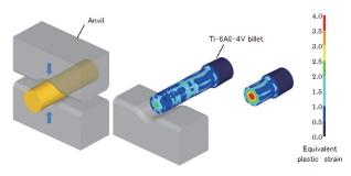
Fig. 5 Distribution of equivalent plastic strain during hot forging calculatated by FEM analysis in Ti-6Al-4V billet
