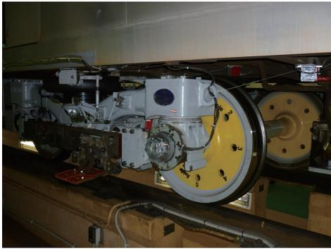
Photo 1 Bogie for wheel/rail contact force measurement
