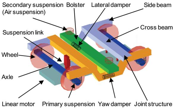
Fig. 4 Simulation model for linear-motor metro bogie
