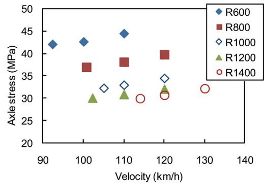
Fig. 14 Relationship between vehicle velocity and axle stress
