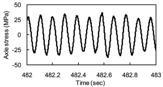
**Fig. 9** Example of measured axle bending stress
