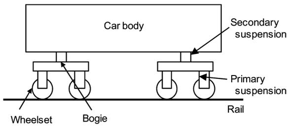
Fig. 1 Configuration of railway vehicle
