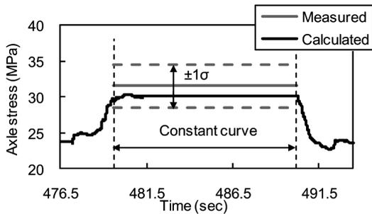
Fig. 12 Transient dynamic analysis of axle stress
