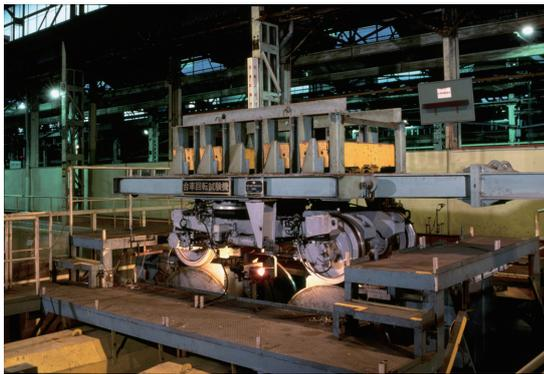
Photo 2 Rotating-disc type test bed for bogie
