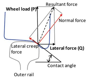
Fig. 3 Contact force between wheel and rail on vertical section
