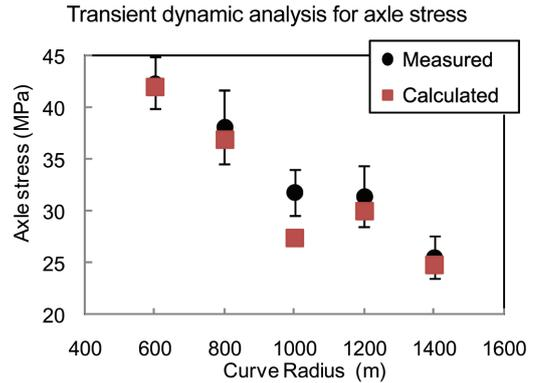
Fig. 13 Comparison of measured and calculated stress
