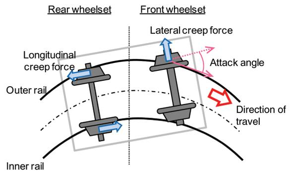
Fig. 2 Bogie behavior during curve negotiation and contact force between wheel and rail
