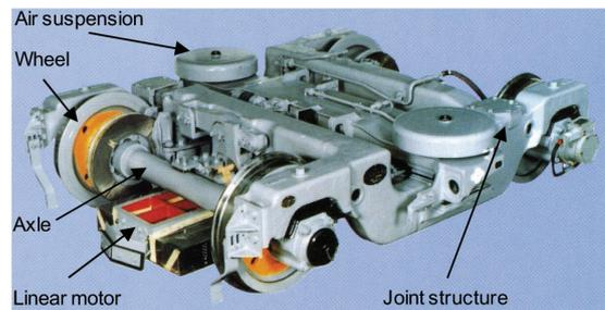
Photo 3 Bogie for linear-motor metro
