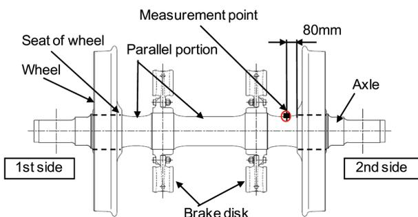
**Fig. 8** Wheelset and stress measurement point
