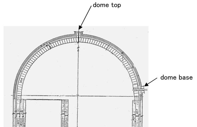
Fig. 4 Observation holes on the dome
