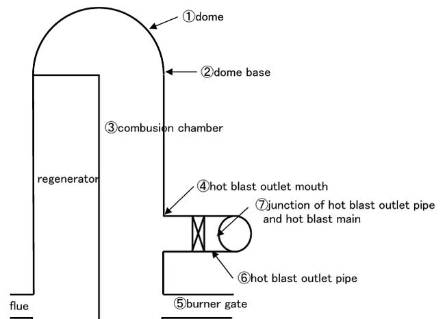
**Fig. 1 Damages in hot-blast stove refractories**
