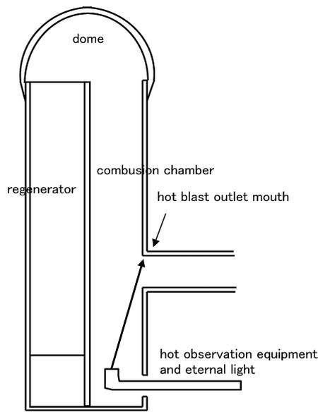
Fig. 7 Observation inside combustion chamber
