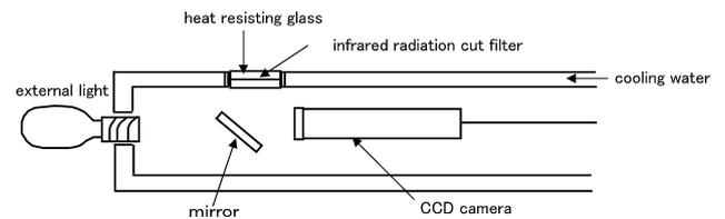
Fig. 5 Hot observation equipment with external light
