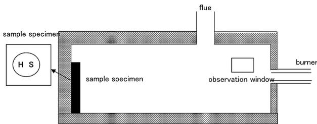
Fig. 2 Test furnace for hot observation
