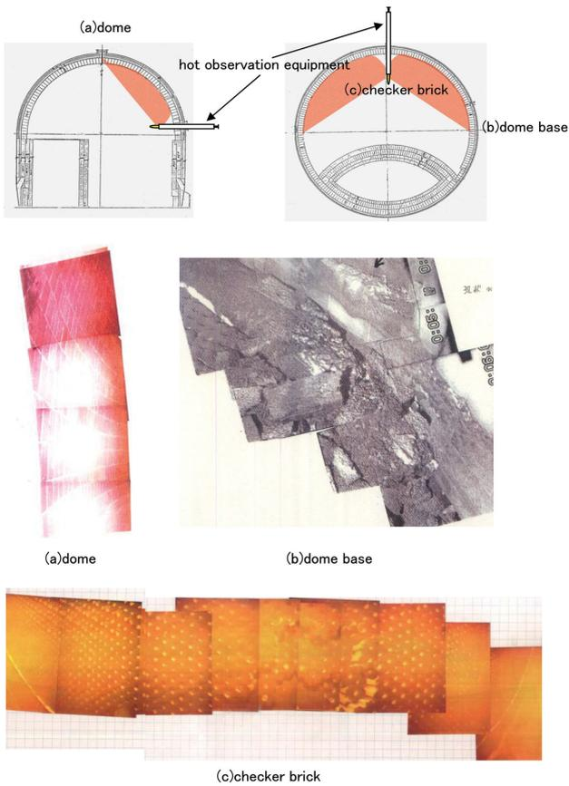
Fig. 6 Obtained images from hot observation inside dome
