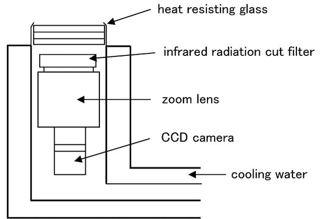
Fig. 8 Hot observation equipment without external light
