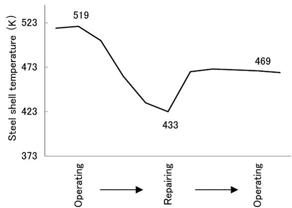
Fig. 14 Temperature of steel shell before and after repair
