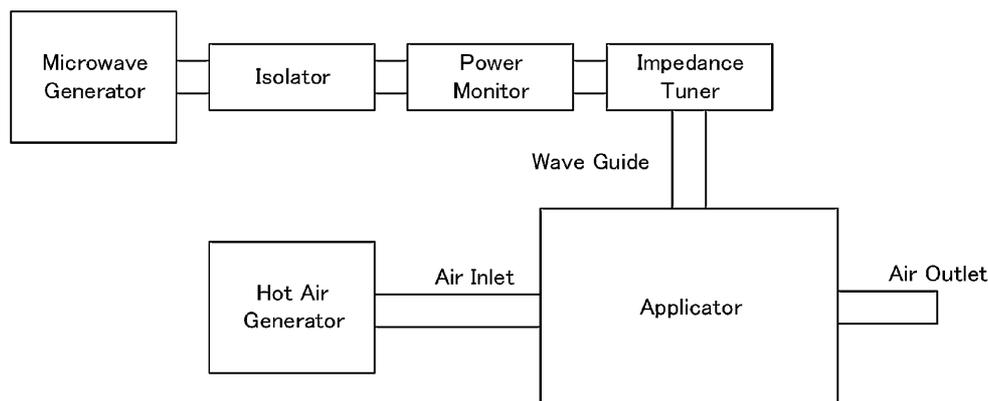
Fig. 3 Microwave drying system
