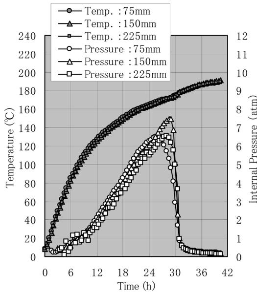
Fig. 6 Temperature and internal pressure in the blocks during microwave drying of alumina-spinel monolithic refractories
