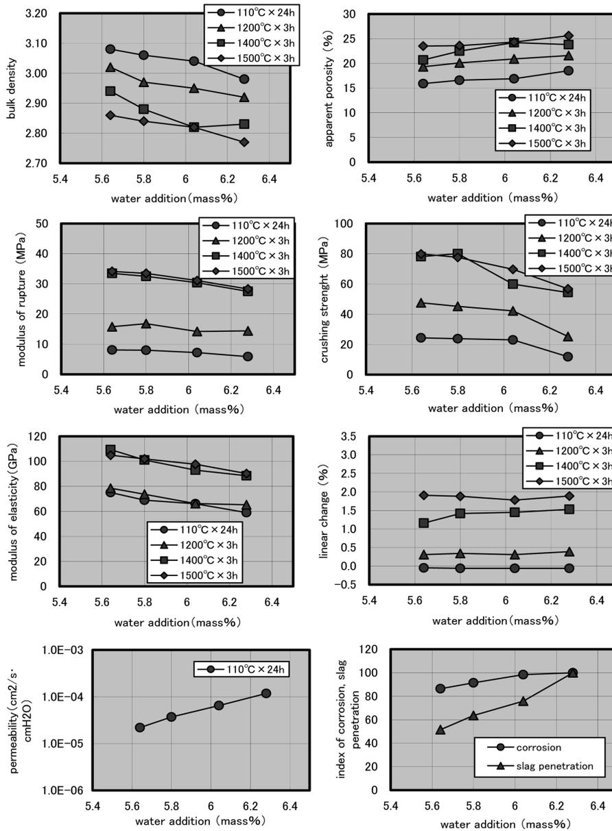
Fig. 5 Relationship between the water addition and some physical and chemical properties
