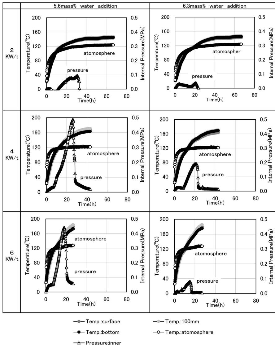
Fig. 4 Temperature and internal pressure in the blocks during microwave drying of alumina-magnesia monolithic refractories
