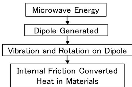
Fig. 2 Principle of microwave heating
