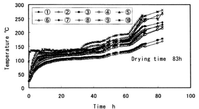
Fig. 11 Temperature change in the lower vessel by new drying pattern
