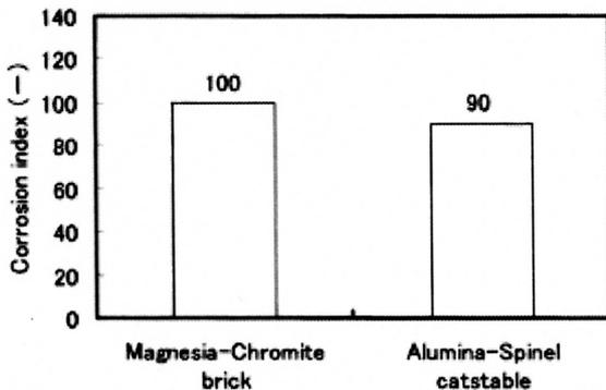
Fig. 12 Results of corrosion test by iron oxide
