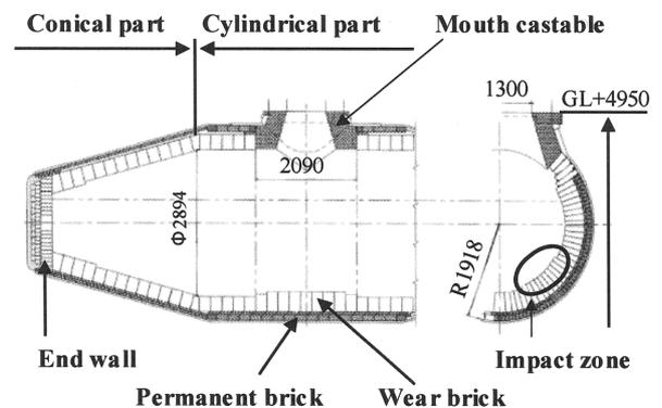
Fig. 1 Lining of torpedo car
