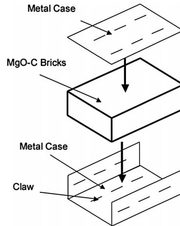
Fig. 8 MgO-C brick with metal case
