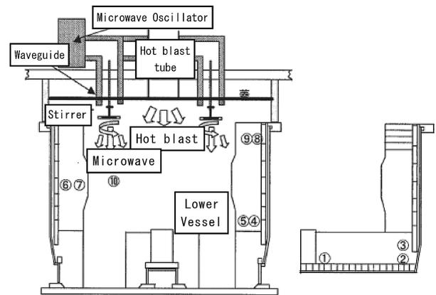
Fig. 10 Temperature measuring points in the lower vessel
