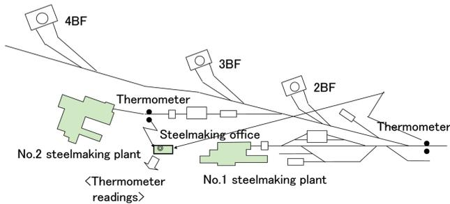
Fig. 5 Measuring system of shell temperature using 2-dimensional thermometers
