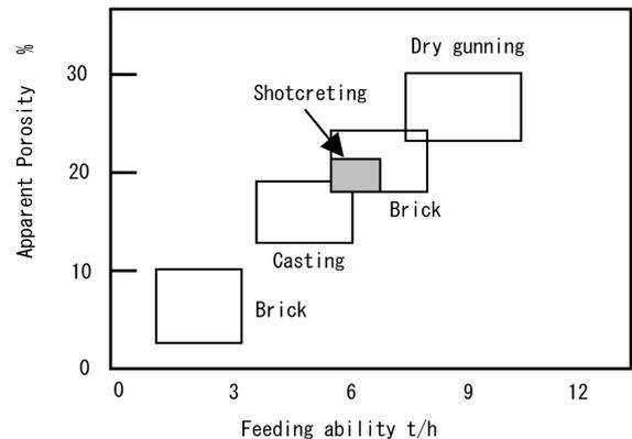
Fig. 14 Comparison of construction methods
