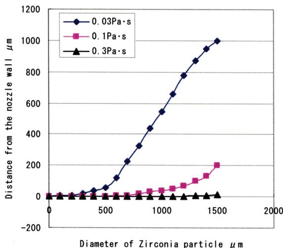
**Fig. 15** Distance of zirconia particles from the nozzle wall as a function of diameter (300cpm)
