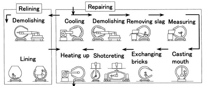
Fig. 2 Item of repairing and relining on using shotcreting
