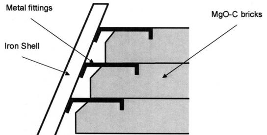
Fig. 7 Brick-fixing structure in the cone of BOF
