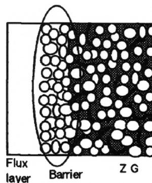
**Fig. 16** Schematic illustration of barrier at nozzle outer surface
