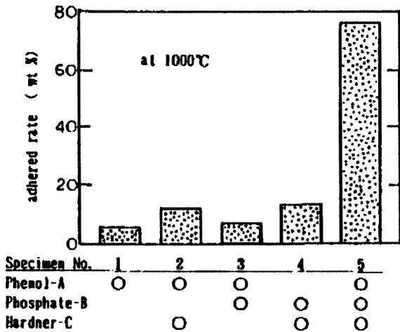
Fig. 9 Relation between combination of binders and adhered rate
