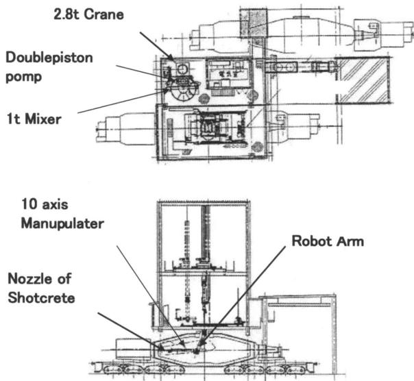
Fig. 4 Automatic shotcreting apparatus
