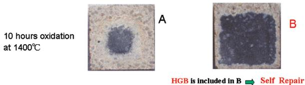
the pores close in the refractory as a result of appropriate sintering progress. Since the refractory is not oxidized any more even when it is reheated, it is considered that the refractory has a self-repairing function.
