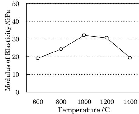
Fig. 21 Modulus of static elasticity of No.2 nanotech magnesia carbon brick
