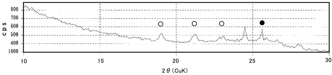
Fig. 19 XRD patterns of a No.1 nanotech magnesia carbon brick after firing at 1,000. Open circles show peaks of  $B_4C$ , and closed circles shows peaks of graphite. Horizontal axis shows  $2\theta$  using copper target, and vertical axis shows intensity respectively.
