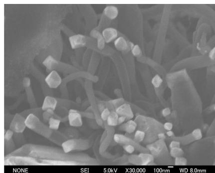
Fig. 13 Fiber like structure in carbonized matrix
