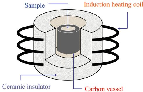
Fig. 2 Induction field activated self-propagating high-temperature synthesis
