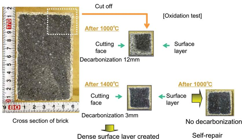
Fig. 17 Oxidation resistance of white MgO-C nanotech refractories
