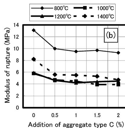
Fig. 8 Additional effect of aggregate C type
