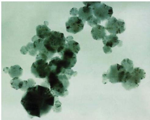
Fig. 3 TEM image of HGB with B<sub>4</sub>C
