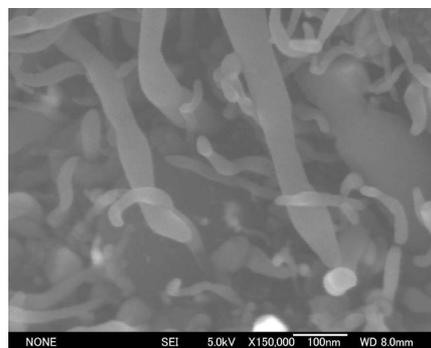
Fig. 12 Lace like structure in carbonized matrix
