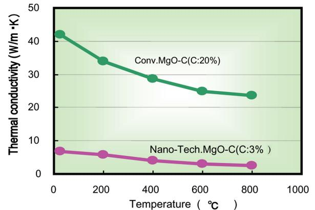
Fig. 9 Thermal conductivity of MgO-C bricks
