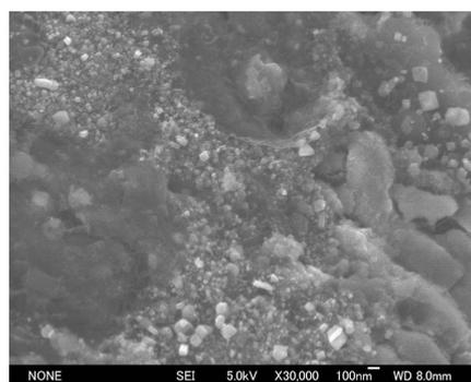
Fig. 11 (a) FE-SEM image of Nano structural matrix of specimen X in Table 3
