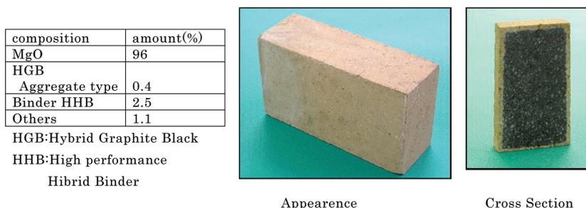
Fig. 15 White MgO-C nanotech refractories (WMC)
