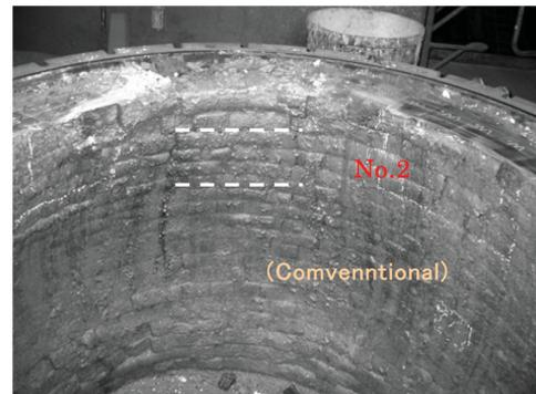
Fig. 22 No.2 nanotech magnesia carbon brick in a RH degasser sidewall after use (between broken lines)
