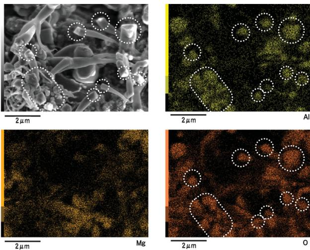
Fig. 14 Composition analysis of fiber like structure
