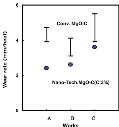
Fig. 10 Performance of nanotech MgO-C brick applied to practical use
