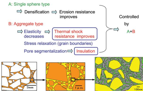
Fig. 6 Effect of nano structural matrix
