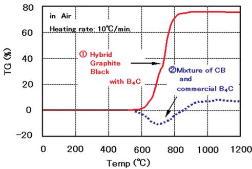
Thermal Gravity Analysis shows Oxidation Behavior in Air
