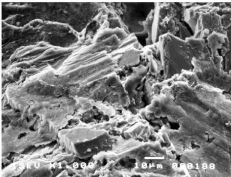
Fig. 20 SEM image of fracture surface of No.1 nanotech magnesia carbon bricks after firing at 1,000
