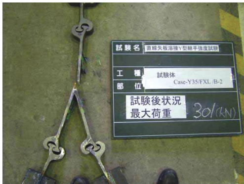
Photo 10 One of the test results in junction of steel sheet pile cell
