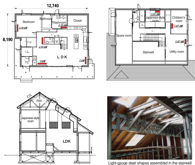
Fig. 7 Summary of Engaru-specification (1st floor plan [upper left], 2nd floor plan [upper right], section [lower left], introspective photo under construction [lower right])
